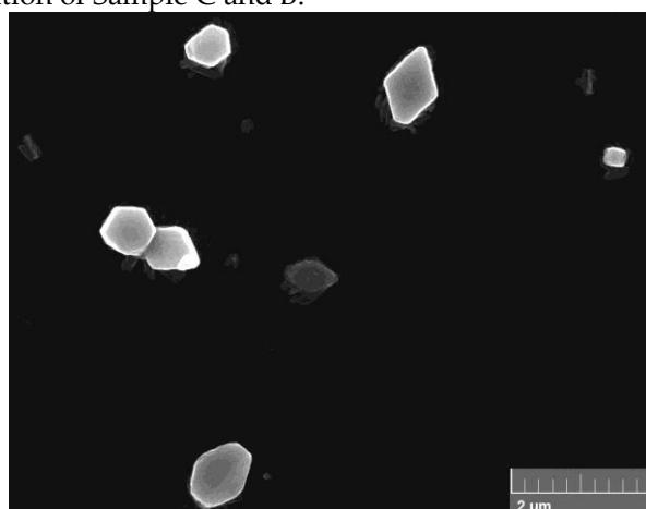
**Figure S1.** SEM analysis of sample A (of 30 nmol of Cd deposited on n-Si) at high magnification.
