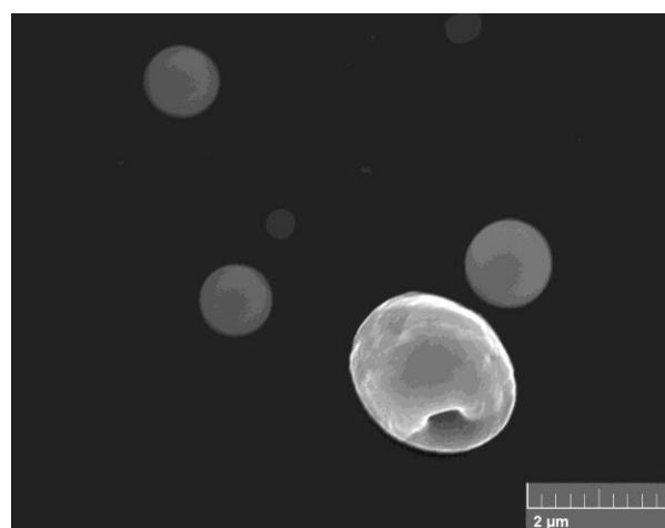
**Figure S2.** SEM analysis of sample B (30 nmol of Se deposited on n-Si) at high magnification.
