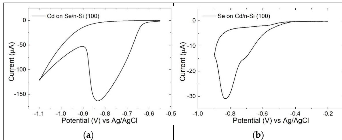
**Figure S3.** a) CV of Cd<sup>2+</sup> solution on Se deposited on n-Si performed between -0.55 V and -0.9 V, scan rate 10 mV/s; b) a) CV of Se(IV) solution on Cd deposited on n-Si performed between -0.9 V and -0.2 V, scan rate 10 mV/s;.
