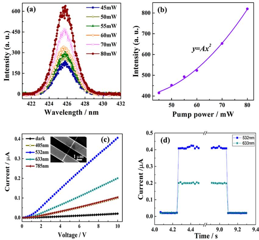
**Figure 16.** (a) Second-harmonic generation spectra of the BNW film under 850-nm illumination with different pump powers. (b) The curves of the second harmonic generation (SHG) peaks' intensity versus the pump powers. (c) The photocurrent-voltage curves of an individual BNW under different irradiations. The inset is the nanodevice structure. (d) The fast on-off curves of the BNW under 532-nm and 633-nm irradiations, respectively [50]. Copyright 2018, Wiley.
