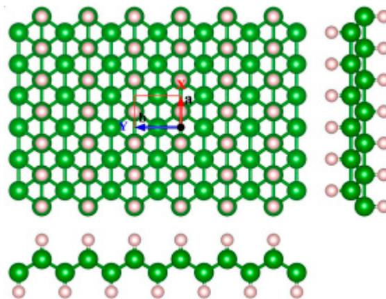
**Figure 9.** Top and side views of the optimized configuration of borophane. The unit cell is marked by a red box, in which the green and white balls respectively represent B and H atoms [64]. Copyright 2016, Royal Society of Chemistry.
