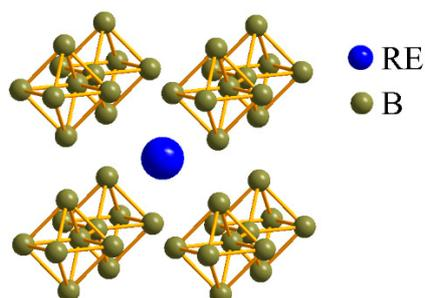
**Figure 1.** Typical lattice structure of rare-earth boride ( $\text{REB}_6$ ).
