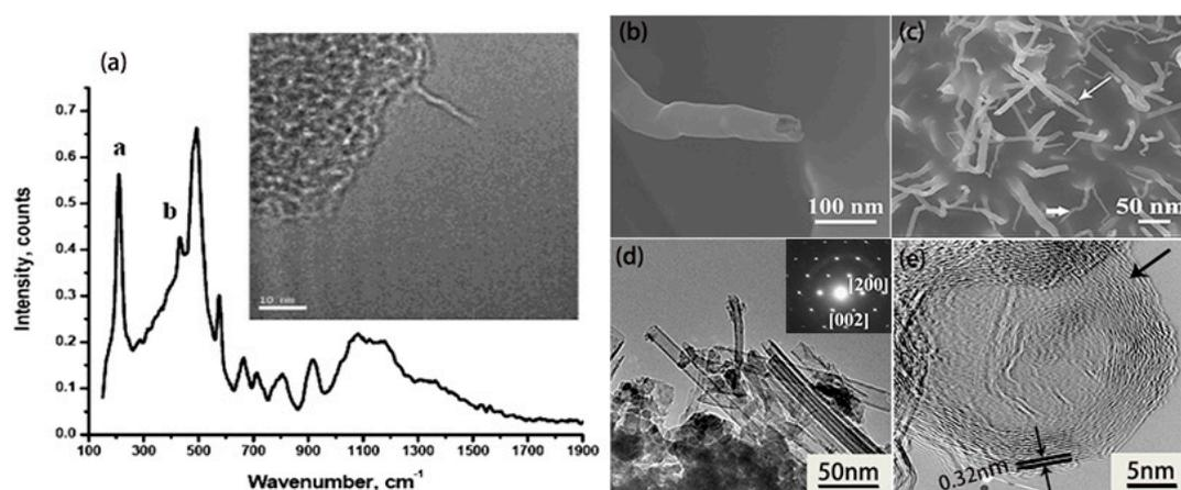
**Figure 4.** (a) Raman spectrum and TEM image (inset) of a single-wall boron nanotube [52]. Copyright 2004, American Chemical Society. (b,c) Low-resolution and high-resolution SEM images of the boron nanotubes (BNTs) (white arrows) at the initial growth stage. (d) TEM image of the BNTs. The inset is the corresponding SAED pattern. (e) The HRTEM image of the top of the BNT [53]. Copyright 2010, Royal Society of Chemistry.
