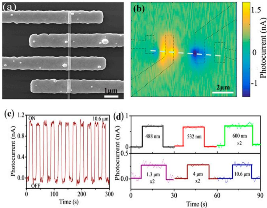
**Figure 17.** (a,b) SEM image and scanning photocurrent mapping of a single SmB<sub>6</sub> nanowire photodetector. (c) The time-dependent photocurrent measurement on the nanowire photodetector under 10.6-μm irradiation. (d) Room temperature photoresponse of the SmB<sub>6</sub> device under photoexcitation with different excitation wavelengths (as marked) [91]. Copyright 2018, American Institute of Physics.
