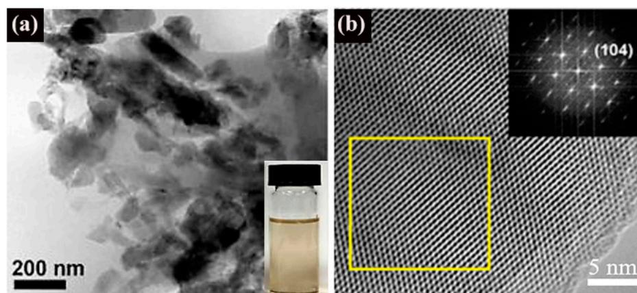
**Figure 8.** (a) Typical TEM images of the few-layer B sheets prepared by tip sonication. The inset is a photograph of B-sheet dispersions and sonication after 4 h. (b) Typical TEM image of the few-layer B sheets. The inset shows the corresponding FFT pattern [62]. Copyright 2018, American Chemical Society.
