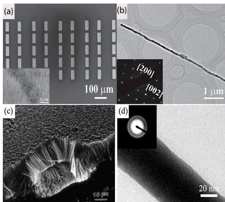
**Figure 3.** (a) Low-magnification SEM images of large area boron nanowire (BNW) arrays, and the inset gives their high-resolution image. (b) Typical HR-TEM image and SAED pattern of the single-crystalline BNW [51]. Copyright 2014, Wiley. (c,d) SEM and TEM image of the amorphous BNWs. Inset, SAED pattern taken from the nanowire showing some amorphous halo rings [46]. Copyright 2001, Wiley.
