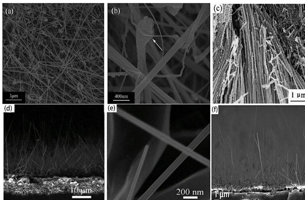
**Figure 2.** (a,b) Typical low-magnification and high-magnification SEM images of the  $\text{PrB}_6$  nanowires [39]. Copyright 2014, Elsevier. (c) Low-magnification SEM images of the  $\text{NdB}_6$  nanowires [41]. Copyright 2013, Elsevier. (d,e) Representative morphologies of the  $\text{LaB}_6$  nanowires [44]. Copyright 2017, Royal Society of Chemistry. (f) Side-view SEM image of the  $\text{SmB}_6$  nanowires [45]. Copyright 2017, IOP Publishing.
