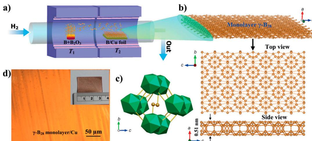
**Figure 7.** (a) Schematic diagram of the two-zone CVD furnace for two-dimensional (2D)  $\gamma\text{-B}_{28}$  film. (b) Top and side views of the borophene monolayer. (c) The corresponding polyhedral structure of the basic unit cell in  $bc$  projection, in which boron atoms (orange spheres) form the dumbbells. (d) Optical image of a monolayer on Cu foil [23]. Copyright 2015, Wiley.
