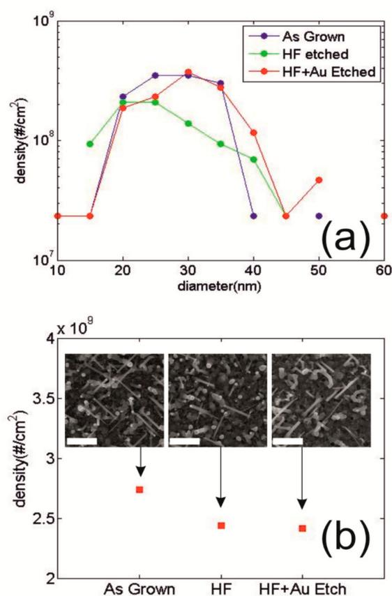
**Figure 3.** (a) Si-NWs density as a function of diameter is reported for as-grown sample (blue circles), after the HF etching (green circles) and after HF + Au etching (red circles). (b) Average Si-NWs surface density for the three cases under study. The inset shows the relative SEM micrograph in planar view scale markers corresponds to 400 nm.
