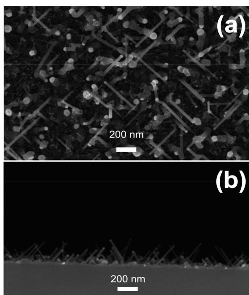
**Figure 1.** Scanning electron microscope (SEM) micrographs in planar (a) and cross-sectional view (b) of silicon nanowires (Si-NWs) array grown on Si (100) substrate, prepared by Au-catalyzed VLS growth in plasma ambient.
