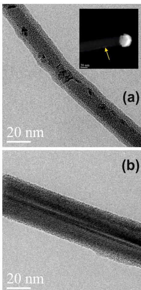
**Figure 6.** (a) TEM micrograph in cross-sectional view of nanowires without any previous gold etching process and annealed by Rapid Thermal Annealing (RTA) at 800 °C for 30 min. The inset shows a STEM image of the same sample. It is clearly visible that Au is present not only on the tip, but also on the NW sidewalls (as indicated by the yellow arrow). (b) TEM micrograph in cross-sectional view of Si-NWs with the double-step gold etching process and annealed by RTA at 800 °C for 30 min.
