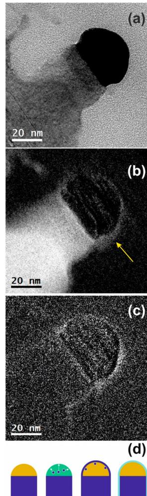
**Figure 2.** Transmission electron microscopy (TEM) micrograph acquired in bright field conditions of a Si-NW on <100> Si substrate (a). Silicon map (b) and oxygen map (c) acquired through energy filtered TEM (EFTEM) analysis on the same nanowire. A thin layer (indicated by the yellow arrow in b) is observed around the metal dot. Schematics illustrating the mechanisms of SiO<sub>2</sub> layer formation around the Si-NWs tip (d).
