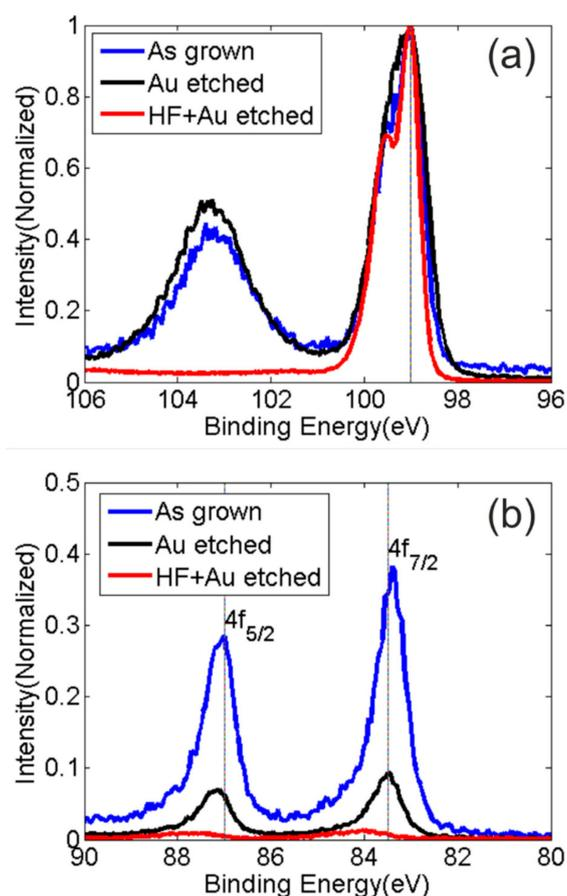
**Figure 5.** High resolution X-ray photoelectron spectra of the (a) Si 2p and (b) Au 4f of the as-grown nanowires (blue line), the sample obtained after the gold etching (black line) and the sample obtained after the two-step procedure (red line).
