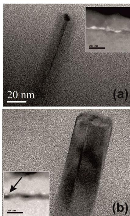
**Figure 4.** Cross-sectional view of TEM micrographs of Si-NWs after the gold removal single step (a), and after the two-step gold etching (b). Insets: STEM micrographs of the substrate/Si-NWs interface for the relative samples.
