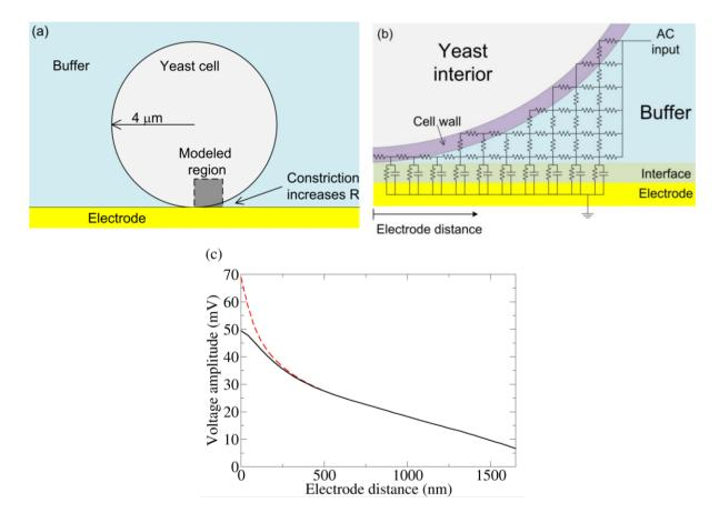
Thus the applied sinusoidal voltage across the two outer electrodes is largely dropped at the electrode interface. This is due to the interfacial capacitance. However, when a cell approaches an outer electrode, the cell-electrode constriction increases the charging resistance near the gap, blocking the electrode from charging underneath the cell. This reduces the voltage at the interface, allowing some of the voltage to be dropped across the cell.
