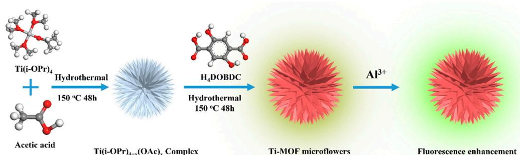
**Scheme 1.** Schematic illustration for manufacturing hierarchical Ti-MOF microflowers and Al(III) ions luminous sensing.
