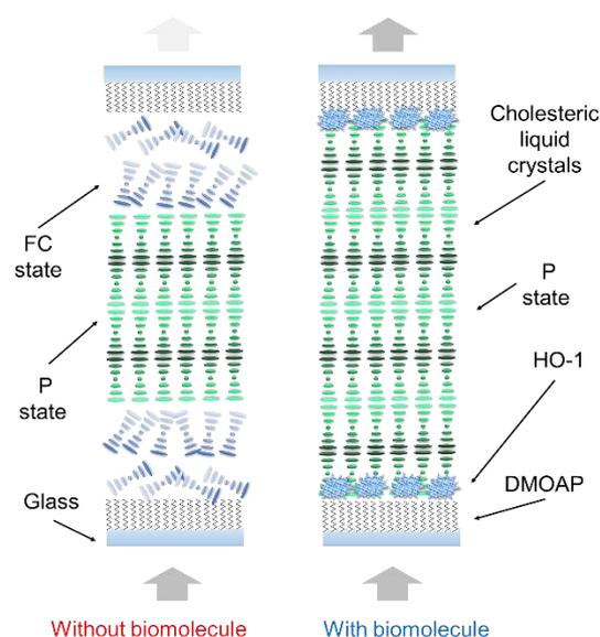
**Figure 1.** Illustration of the cholesteric liquid crystal (CLC) biological sensor chip in the presence of heme oxygenase (HO)-1 biomolecules in the DMOAP-coated cell. Different color arrows indicate the different light penetration intensities.
