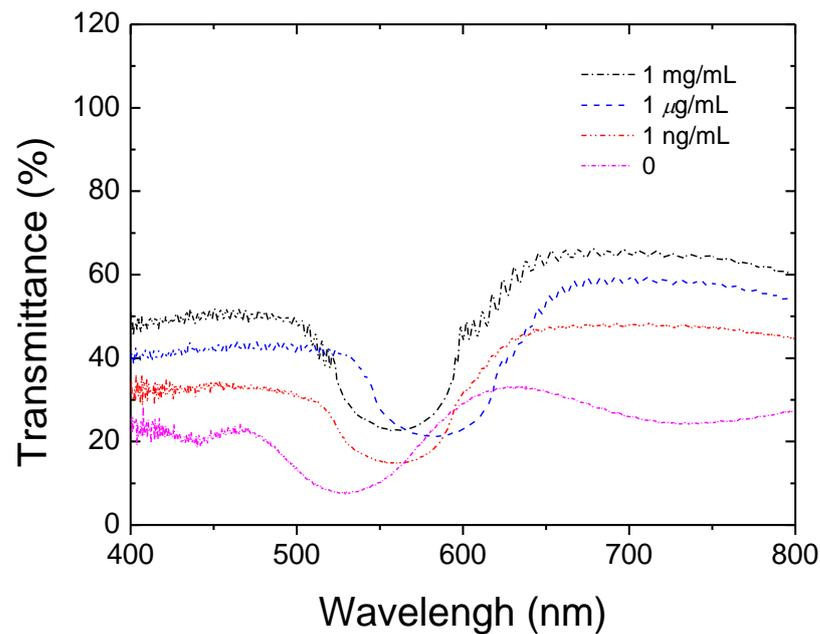
**Figure 3.** Spectra of the cholesteric liquid crystal (CLC) biological sensor immobilized with various concentrations of heme oxygenase (HO)-1 (0~1 mg/mL).
