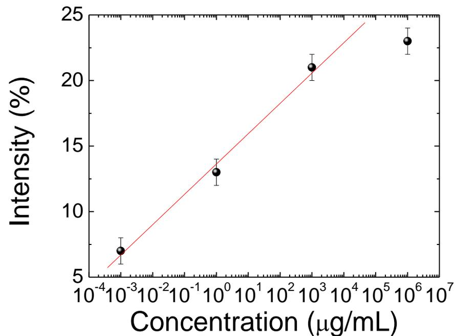
**Figure 4.** Linear positive correlations of the minimum transmittance of the photonic band of the cholesteric liquid crystal (CLC) biological sensor at different heme oxygenase (HO)-1 concentrations.
