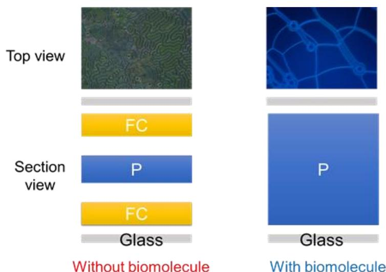
**Figure 2.** Optical mechanism and structure design of the cholesteric liquid crystal (CLC) biosensor both with and without the presence of biomolecules.
