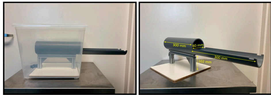
Figure 2. Acclimation Chamber. The simulated acclimation core was cut from PVC pipe and measures 600 mm in total length (300 mm for the core and 300 mm for the open extension). The width of the PVC pipe was 80 mm and the entire core was elevated 102 mm off the platform by a steel rack. The core was designed to mimic a small animal MRI core so that animals acclimated using this structure would exhibit lower stress signals and perform fewer and less drastic head movements during scans.
