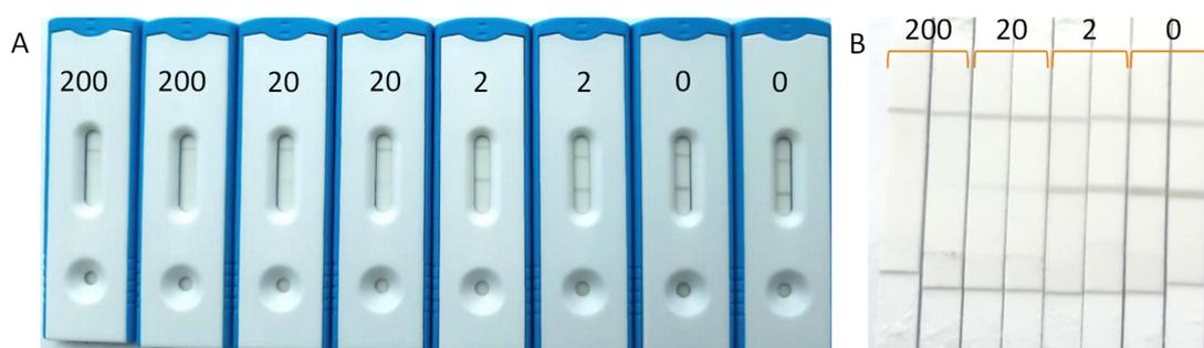
**Figure 4.** Surface water from a brook (Wageningen, The Netherlands) fortified with CHLP at 200, 20, 2, and  $0 \mu\text{g/L}$  and applied to the LFIA in duplicate. Visual imaging was performed in the assembled cassettes (A) and with strips removed from the cassettes for digital imaging (B).
