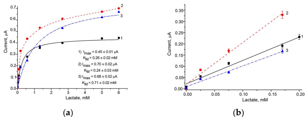
**Figure 5.** Calibration curves of the  $Fcb_2/AuHCF/GE$ s in the broad (a) and linear (b) ranges of the dependence of enzyme quantity on the surface of GE; lines 1, 2, 3 correspond to 13, 25 and 50 mU of  $Fcb_2$ , respectively. The working potential is  $-75$  mV.
