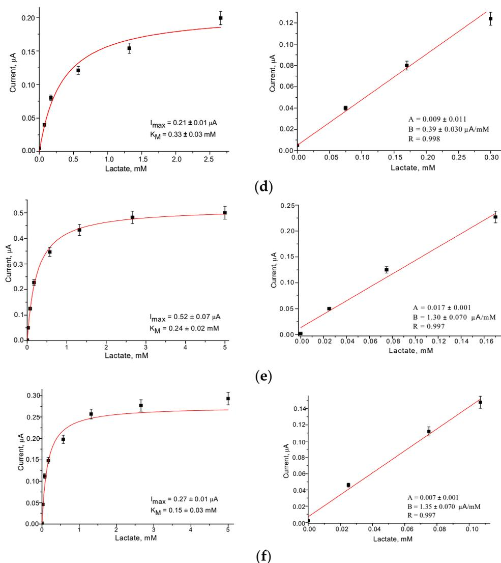
**Figure 4.** Calibration curves for Lact determination in wide (left) and linear (right) ranges using the  $Fcb_2$ /NPs/GEs: (a) control, without NPs; (b–f) samples with AuHCF (b), PdHCF (c), PtHCF (d), PtZn (e), and NiPtPd (f). Each bioelectrode contained 25  $\mu$ M of  $Fcb_2$  and 1  $\mu$ g of NPs on the surface of the GE. Conditions: 50 mM phosphate buffer, pH 8.0, and working potential of  $-75$  mV.
