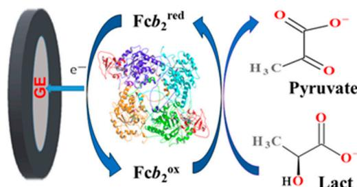
**Figure 1.** The principal scheme of Lact determination using the *Fcb*<sub>2</sub>-based ABS.
