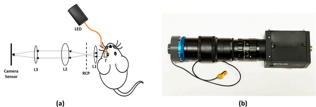
**Figure 2.** (a) The schematic illustration of the experimental setup. (b) Photographic illustration of the imaging system. RCP: Retina conjugate plane.
