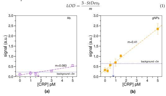
**Figure 7.** Estimation of LOD. (**a**): LOD measured for LFT performed with pure a-CRP-HRP; (**b**): LOD measured for LFT with the functionalized gNPs.
