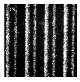
**Figure 4.** Dielectrophoretic bacterial concentration. While sample solution flows past the electrodes, the total donor fluorescence signal, summed over the entire image, from SYTO<sup>®</sup>-9 labeled bacteria (no acceptor is present) increases linearly over time, measuring more than  $400 \times (458.5 \pm 18.2 \times, n = 6)$  the initial value after one minute flow at  $100 \mu L/min$ .
