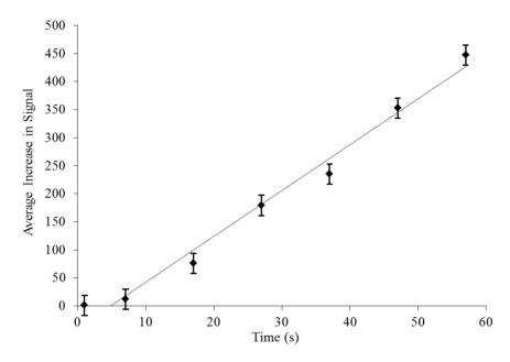
**Figure 5.** Concentration of serial bacterial dilutions after sixty seconds of dielectrophoresis (DEP). Signal increases with initial bacterial concentration in the range of  $10^1$ – $10^6$  cfu/mL.
