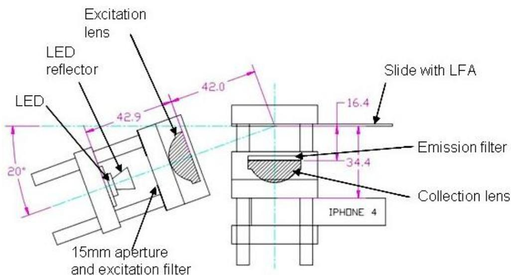
The scattered emission light was first filtered using a single 0.003" thick plastic film (Supergel #15 Deep Straw, Rosco) along with a 2 mm thick, Schott OG570 colored glass filter (FGL570, Thorlabs). The emission light was semi-collimated using a 25 mm diameter, 25 mm FL acrylic lens (NT48-170, Edmund Optics) for collection using the smartphone (iPhone 4). Apertures were hand cut out of black plastic and the system was shielded from room light using a hand fabricated black foam core box.
