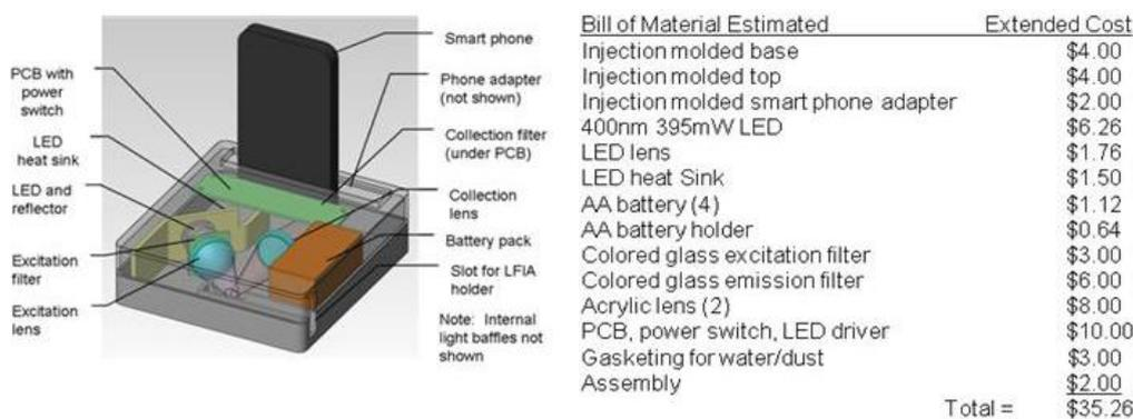
Our ultimate goal is to create a manufacturable reader system that would be an accessory to a smartphone. Shown in Figure 5 is an early concept of such a reader; we have estimated the final cost based on the component parts.
