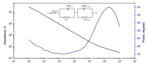
**Figure 2.** Bode plot of a GMEA with an electrode diameter of 20  $\mu$ m. A linear dependency of the impedance at lower frequencies is typical of graphene electrode behavior. The inset gives the model used for fitting the data.
