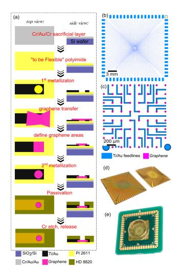
**Figure 1.** (a) Overview of the graphene microelectrode (GMEA) fabrication protocol; (b,c) chip design; (d) optical images of the chip before (left) and after (right) Cr etch; (e) optical image of a flexible chip, which is soldered to a carrier and encapsulated for in vitro stability.
