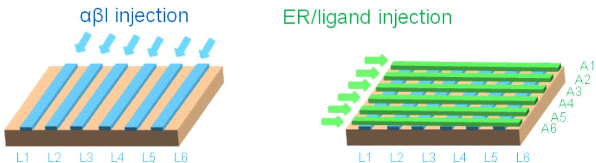
**Fig 1S.** Layout of the NLC chip surface, showing the vertical and horizontal direction for the injection of the  $\alpha\beta$ /I peptide and ER/ligand, respectively.
