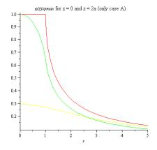
**Graph 1:**  $\varphi/\varphi_{max}$  as a function of r/a for z = 0 (case A, red; case B, green) and z = 2a (case A, yellow).
