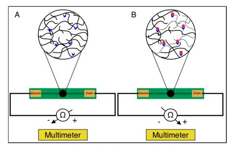
**Figure 2.** Sensing mechanism of the developed biosensors predicated on the electrical percolation principle with (**A**) The biosensor's SWCNT (**black**) and antibody (**blue**) network prior to the addition analyte and (**B**) the biosensor's SWCNT-antibody network following the addition of analyte (**red**), leading to an increase in resistance. Gray SWCNTs are those that are no longer connected in a conductive SWCNT pathway due to the presence of analyte.
