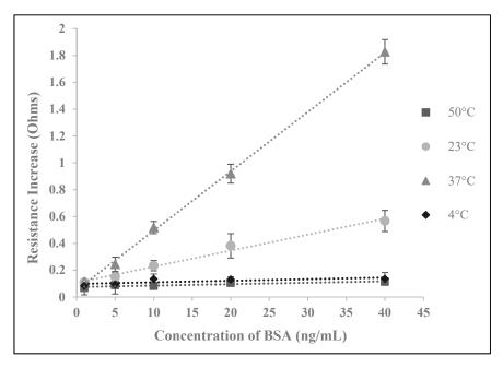
**Figure 4.** Temperature optimization of the sensing conditions for BSA. Biosensors were tested with various concentrations of BSA at 4 different temperatures.
