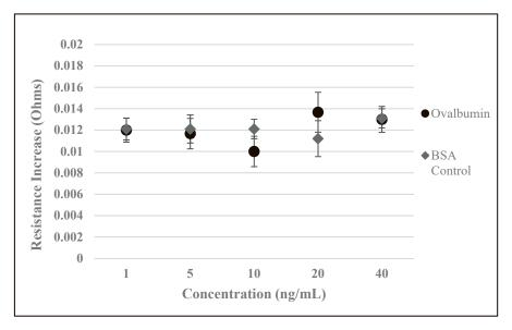
**Figure 5.** Control experiments with the developed biosensors. Developed biosensors were tested with various concentrations of a non-target analyte, ovalbumin. Biosensors were also developed without the use of BSA antibody and tested with various concentrations of BSA.
