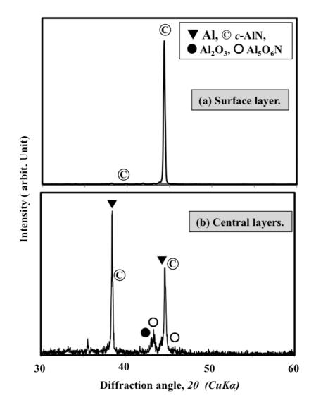
Figure 2. XRD spectra of the fabricated coatings with only Al powder: (a) surface layers and (b) central layers.
