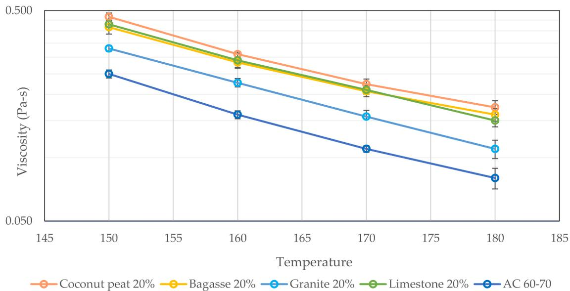
**Figure 5.** The viscosities of asphalt binder and asphalt mastics at 20 rpm with different temperatures.
