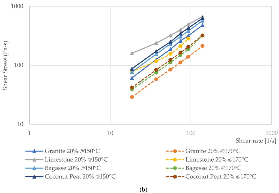
**Figure 4.** The relationship of asphalt mastic (a) viscosity and shear rate and (b) shear stress and shear rate at 150 and 170 °C.
