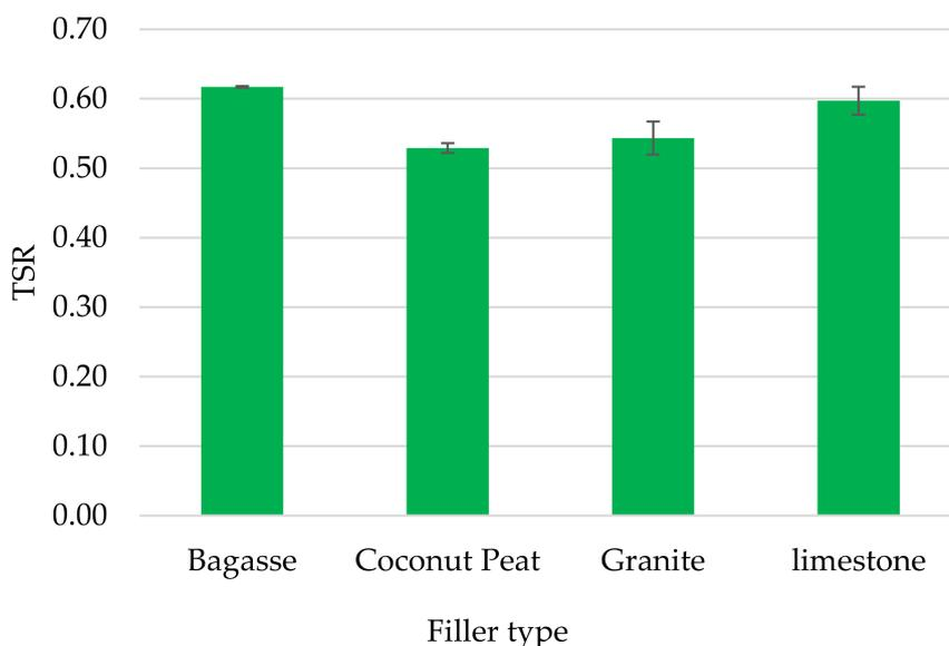
**Figure 7.** TSR of ITS test after moisture of asphalt mixtures with granite aggregate for all filler types.
