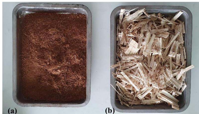
Figure 1. Waste natural materials (a) coconut peat and (b) bagasse.
