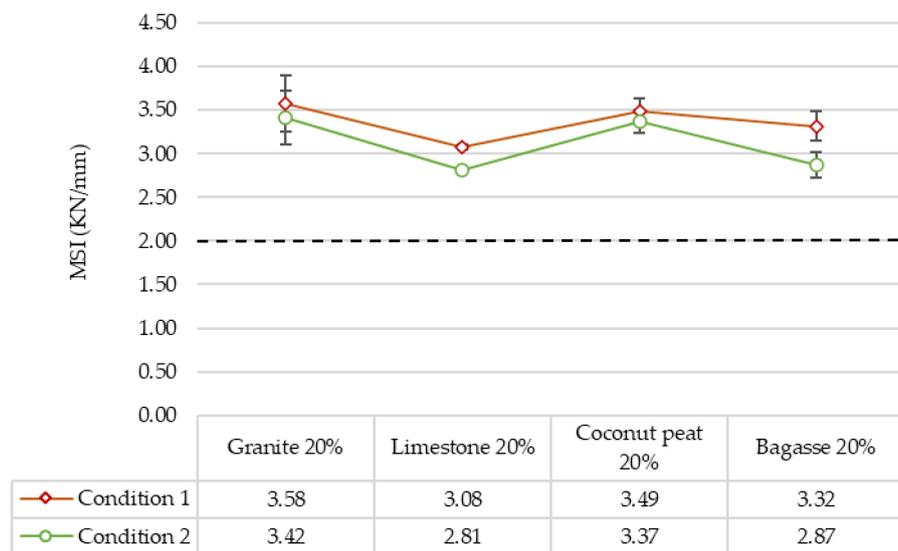
Figure 6. Marshall Stiffness Index of asphalt mixtures.
