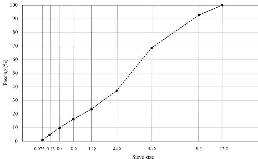
Figure 2. Aggregate gradation.
