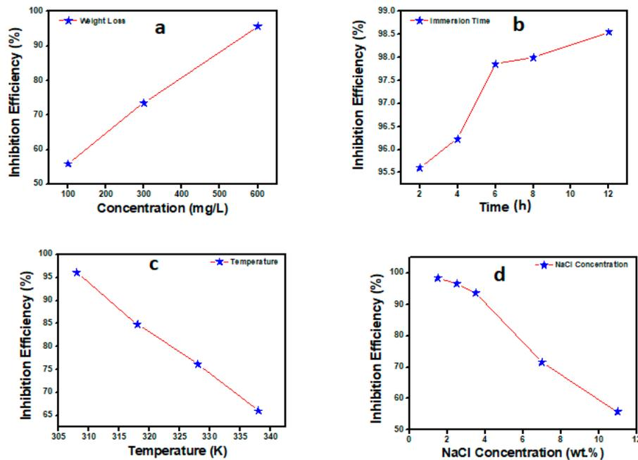
**Figure 3.** (a) Variation of inhibition efficiency (%) with inhibitor concentration. (b) Variation of inhibition efficiency (%) with immersion time. (c) Variation of inhibition efficiency (%) with temperature. (d) Variation of inhibition efficiency (%) with NaCl concentration.
