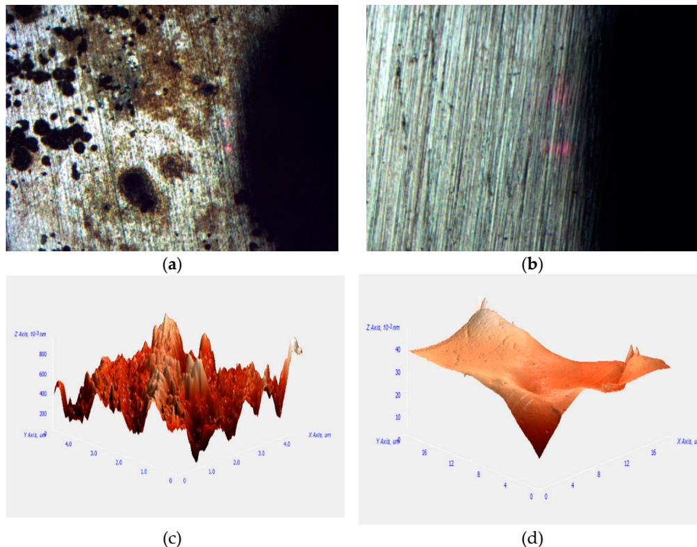
**Figure 9.** Optical image (a) copper surface in a 3.5% NaCl solution (b) copper surface coated with GG-AMPS in a 3.5% NaCl solution; AFM images (c) copper surface in a 3.5% NaCl solution (d) copper surface coated with GG-AMPS in a 3.5% NaCl solution.
