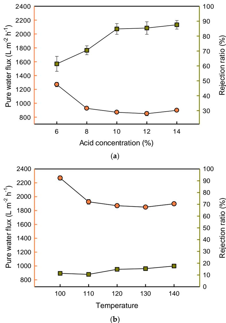
**Figure 4.** Pure water flux and rejection ratio of the composite membrane by acid-curing and heat-curing, respectively (a) Effect of hydrochloric acid concentration on the membrane performance (b) Effect of temperature on the membrane performance.
