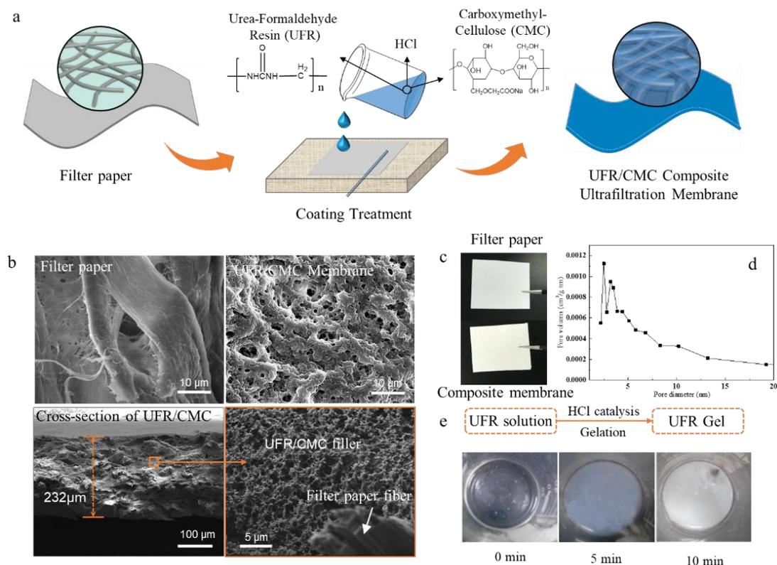
**Figure 1.** (a) Schematic illustration of preparation of the UFR/CMC composite ultrafiltration membrane (b) morphological images of the UFR/CMC composite ultrafiltration membrane (c) photos of filter paper and the composite ultrafiltration membrane (d) pore diameter distribution of the composite ultrafiltration membrane (e) changes in UFR gel degree over time with the addition of hydrochloric acid.
