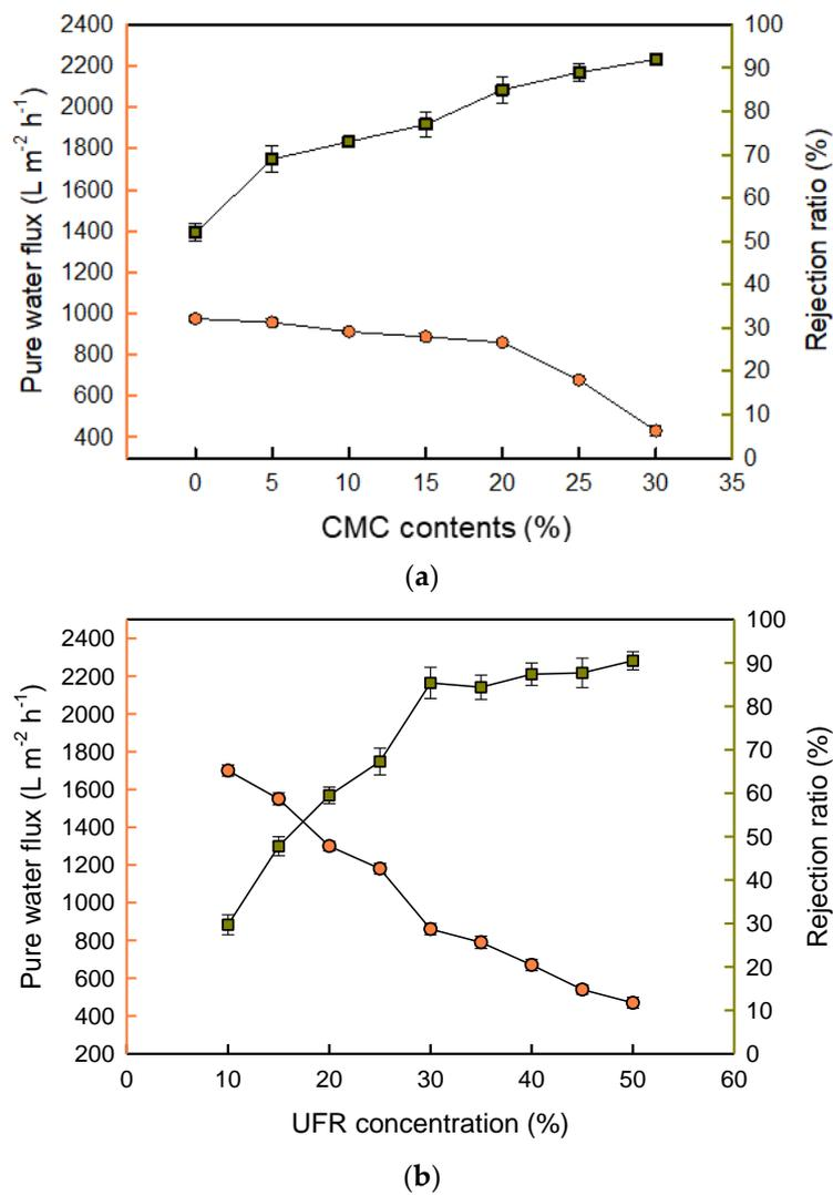
**Figure 2.** Effects of (a) CMC content and (b) urea-formaldehyde resin concentration on the pure water flux and rejection ratio of the composite membrane.
