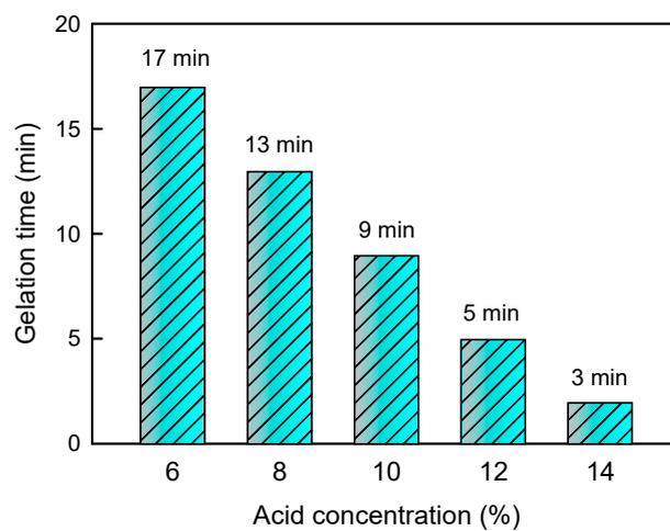
**Figure 3.** Effect of hydrochloric acid concentration on the gelation time of the composite membrane.
