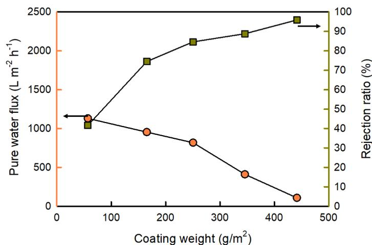
**Figure 5.** Effects of coating weight on the pure water flux and rejection ratio of the composite membrane.
