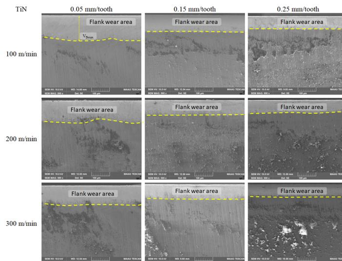
Figure 5. SEM micrographs of flank face for TiN-coated inserts after cutting length of 2800 mm was used for milling.
