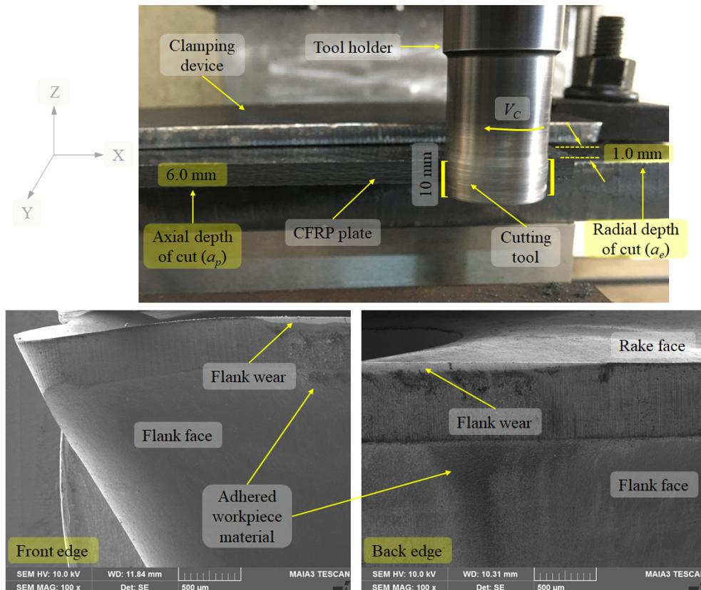
**Figure 11.** Milling conditions and SEM image of cutting tool front and back edge.
