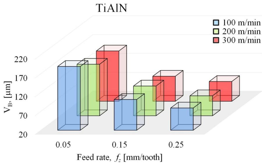
Figure 2. Maximum flank wear of TiAlN-coated inserts as a function of feed rate.
