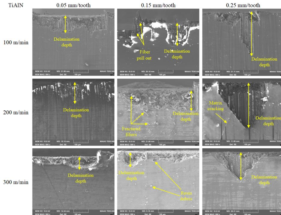
Figure 7. SEM images of CFRP delamination depths at different machining parameters.
