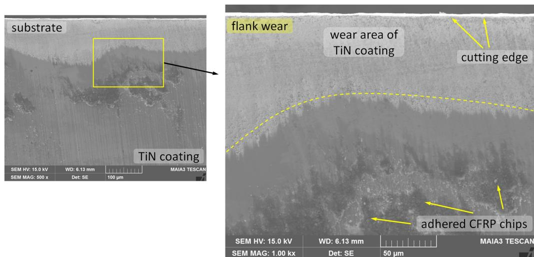
**Figure 17.** SEM micrograph of the deformed TiN-coated insert profile.
