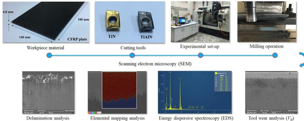
**Figure 1.** Machinability test and representation of the whole experimental set-up.
