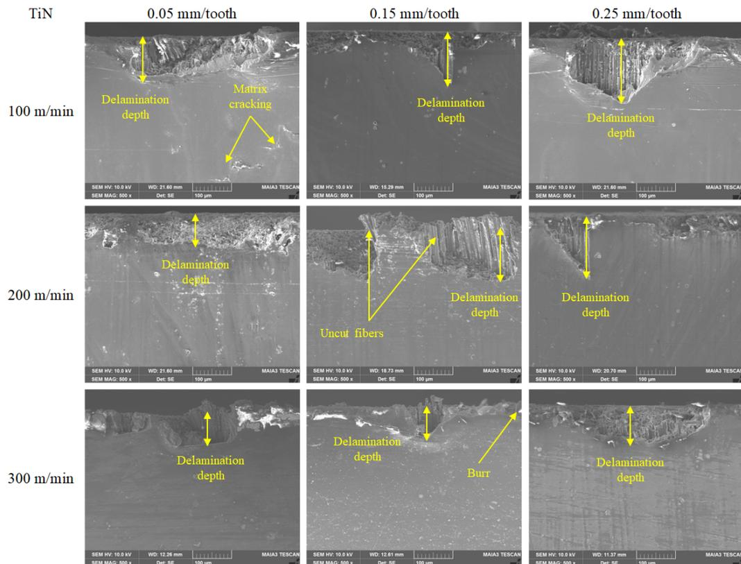
**Figure 9.** SEM images of CFRP delamination depths at different machining parameters.
