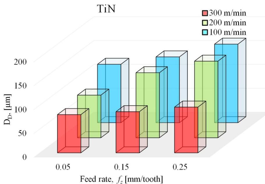
Figure 8. Influence of the machining parameters on delamination depth in the case of TiN-coated inserts.
