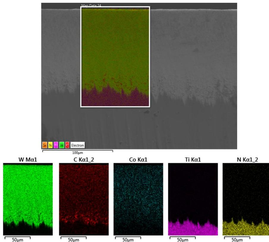
**Figure 14.** SEM micrographs and elemental mapping of the maximum worn TiN-coated insert.
