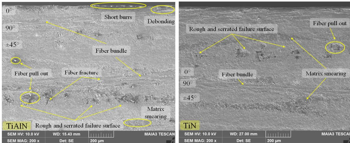
**Figure 10.** SEM images of CFRP surface after machining with TiAlN- and TiN-coated inserts, at 0.25 mm/tooth feed rates and after using the cutting length of 2800 mm.
