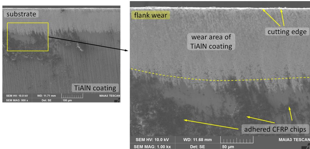
**Figure 16.** SEM micrograph of the deformed TiAlN-coated insert profile.
