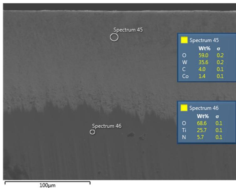
**Figure 15.** SEM micrographs and EDS analysis of the maximum worn TiN-coated insert.
