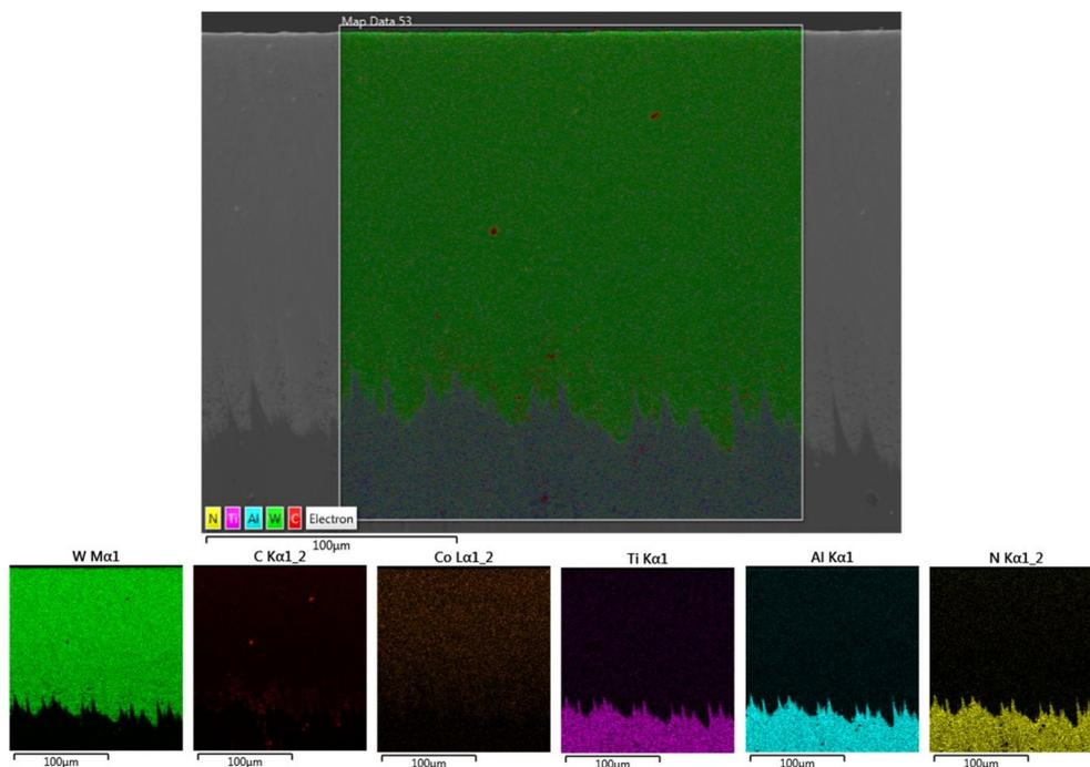
**Figure 12.** SEM micrographs and elemental mapping of the maximum worn TiAlN-coated insert.
