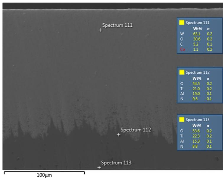
**Figure 13.** SEM micrographs and Energy Dispersive Spectroscopy (EDS) analysis of the maximum worn TiAlN-coated insert.
