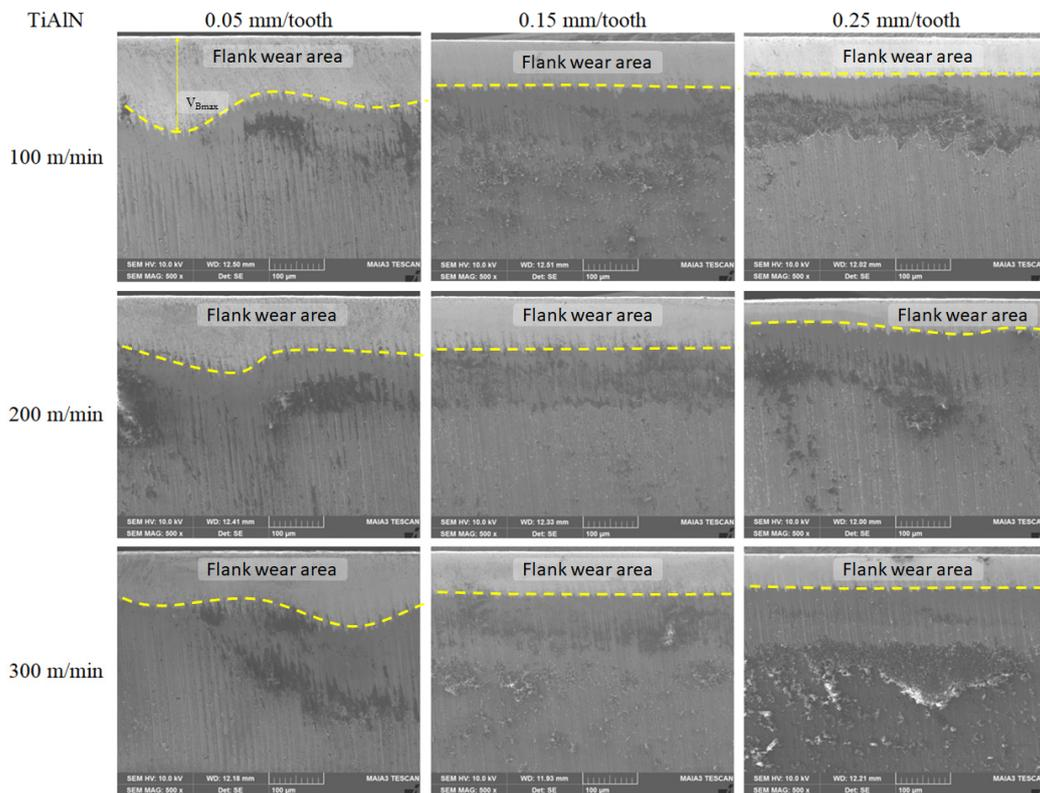
Figure 3. Scanning Electron Microscope (SEM) micrographs of flank face for TiAlN-coated inserts after cutting length of 2800 mm was used for milling.
