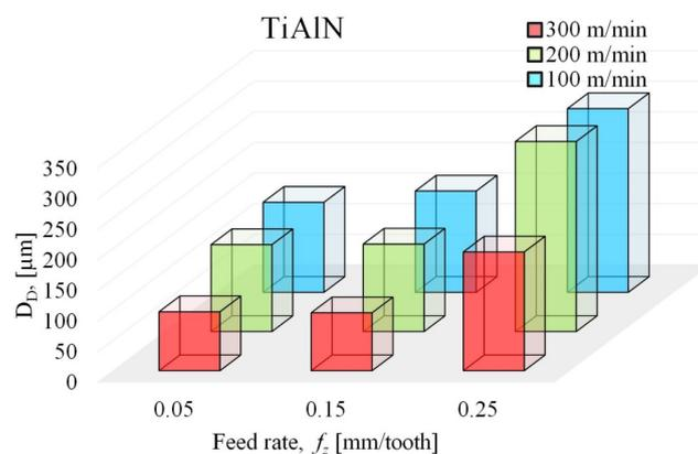
Figure 6. Influence of the machining parameters on delamination depth at TiAlN-coated inserts.
