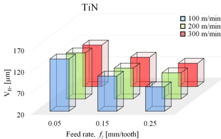
Figure 4. Maximum flank wear of TiN-coated inserts as a function of feed rate.
