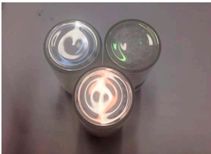
**Figure 1.** Silica-based photonic glass with various colors.
