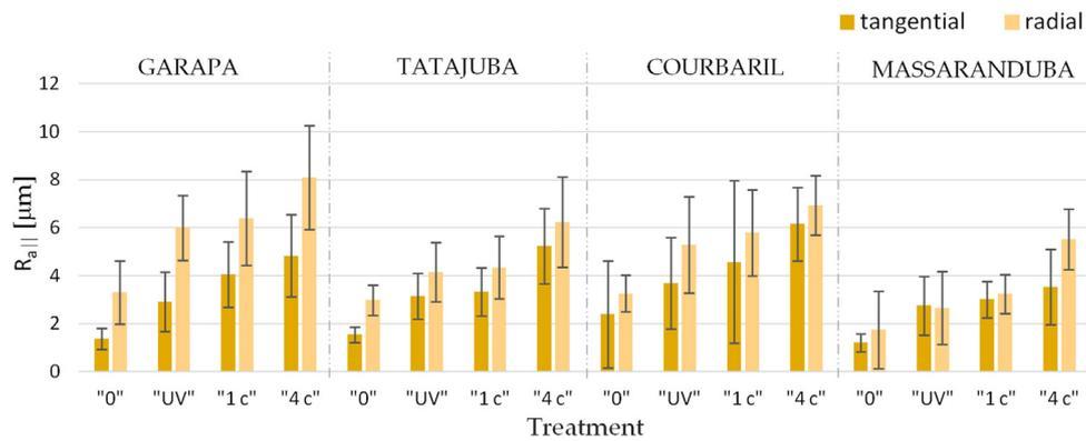
**Figure 2.** Roughness ( $R_{aII}$ ) along the fibres of tested wood species: "O"—fresh wood, "UV"—after 24 h of UV irradiation, "1 c"—after one cycle of artificial weathering, "4 c"—after four cycles of artificial weathering.
