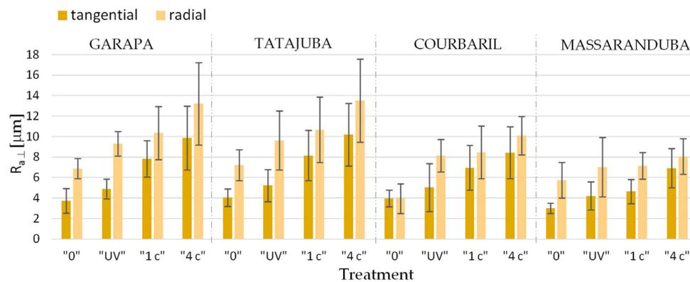
**Figure 3.** Roughness ( $R_{aI}$ ) perpendicular to the fibres of tested wood species: "O"—fresh wood, "UV"—after 24 h of UV irradiation, "1 c"—after one cycle of artificial weathering, "4 c"—after four cycles of artificial weathering.
