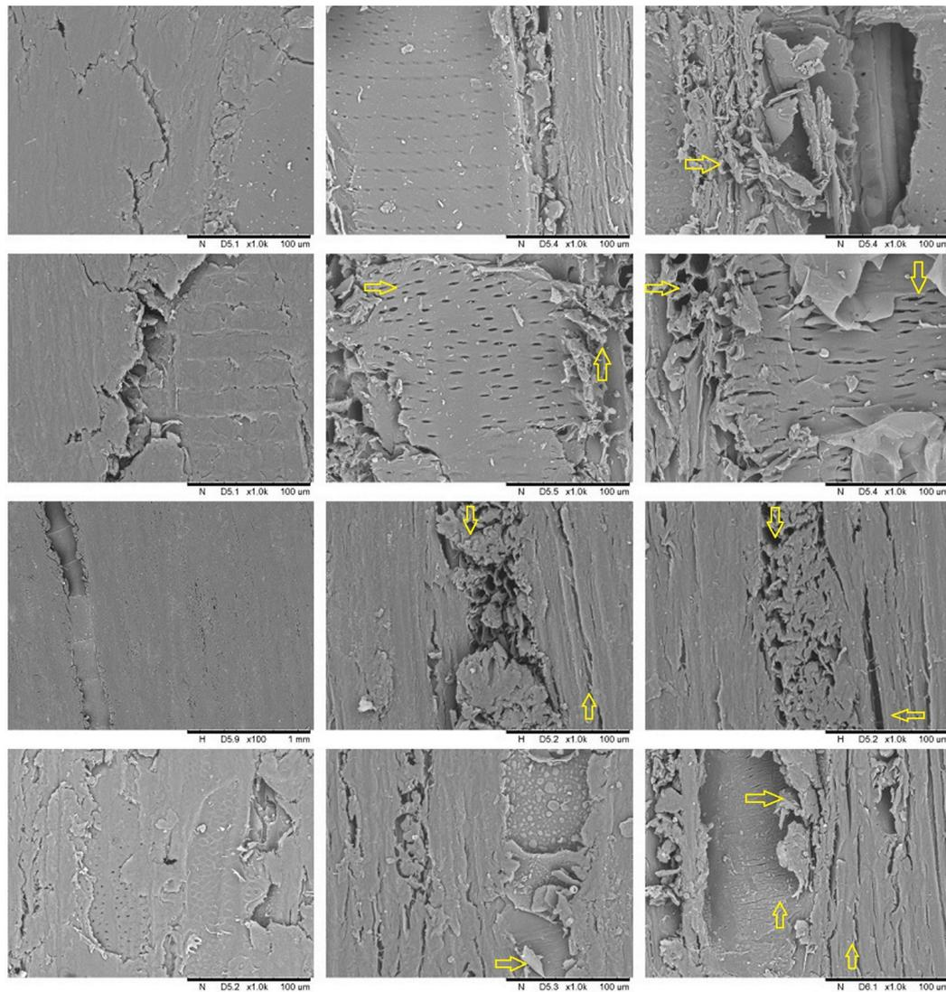
**Figure 4.** Comparison of microstructure exposed and non-exposed wood surface (from top: garapa, tatajuba, courbaril and massaranduba; from left: fresh wood, after 24 h of UV irradiation, after 4 cycles of artificial weathering); the described changes are marked with yellow arrows.
