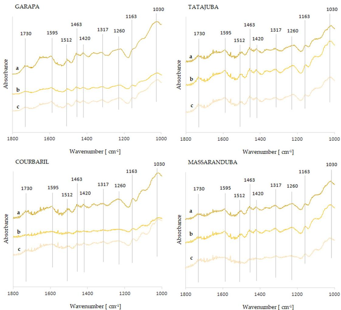
**Figure 5.** FTIR spectra of tested wood species before, after UV irradiation and after four full artificial weathering cycles: **a**—fresh wood, **b**—after UV irradiation, **c**—after four artificial weathering cycles.
