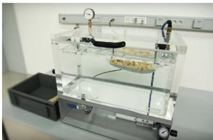
Figure 10. Leak detection by Leak Master Easy ® device, reprinted with permission from WITT Polska.
