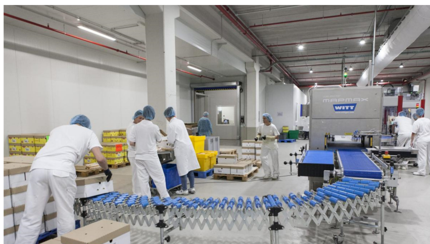
Figure 13. Non-destructive 100% control of packaging tightness, in-line device Leak Master MAPMAX ® , reprinted with permission from WITT Polska.
