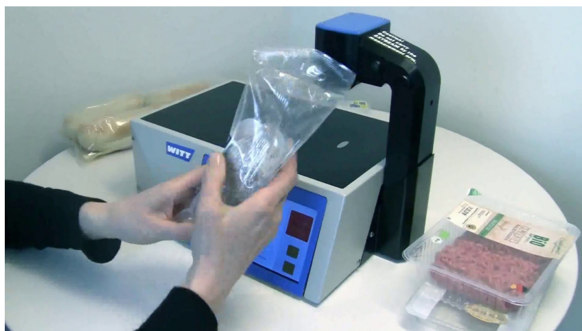
Figure 9. Non-destructive method of O 2 or CO 2 measurement by Oxybeam ® analyzer, reprinted with permission from WITT Polska.
