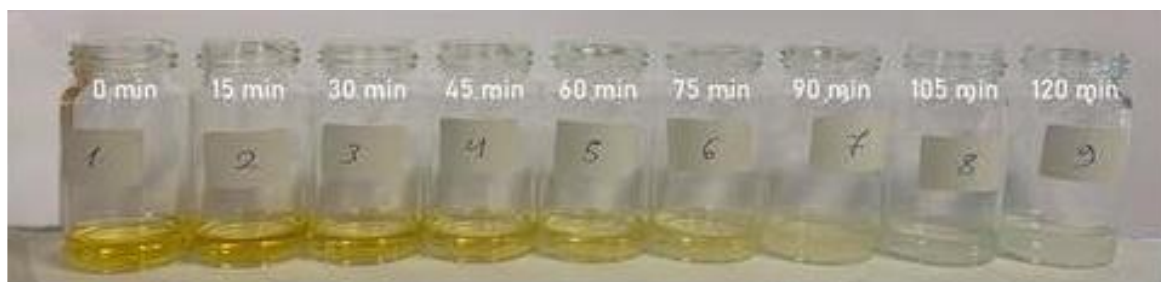
Figure S4. \text{TiO}_2/\text{C-dots} : Macroscopic image of Methylene Orange photodegradation by Vis.
