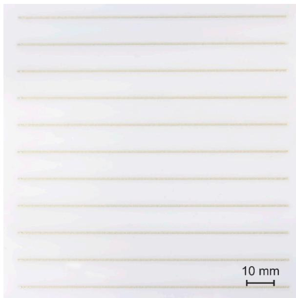
**Figure 2.** Photography of samples used: polycarbonate substrate with 11 printed conductive lines produced from silver paste 1901-SB. Length of each line is 100 mm, width of each line is approximately 0.75 mm, cross-section before curing is approximately  $0.055\text{ mm}^2$ .
