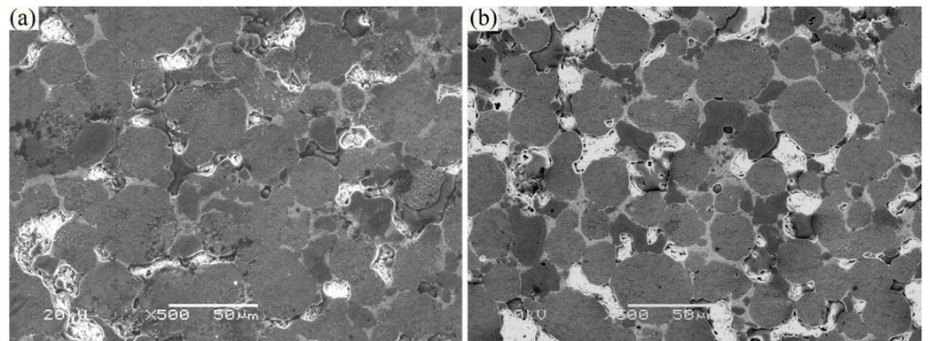
**Figure 2.** The SEM images of CoCrFeNiMn-Cr<sub>3</sub>C<sub>2</sub>-Ag-CaF<sub>2</sub>/BaF<sub>2</sub> composites: (a) CoCrFeNiMn-Cr<sub>3</sub>C<sub>2</sub>-Ag-5%CaF<sub>2</sub>/BaF<sub>2</sub>, and (b) CoCrFeNiMn-Cr<sub>3</sub>C<sub>2</sub>-Ag-15%CaF<sub>2</sub>/BaF<sub>2</sub>.
