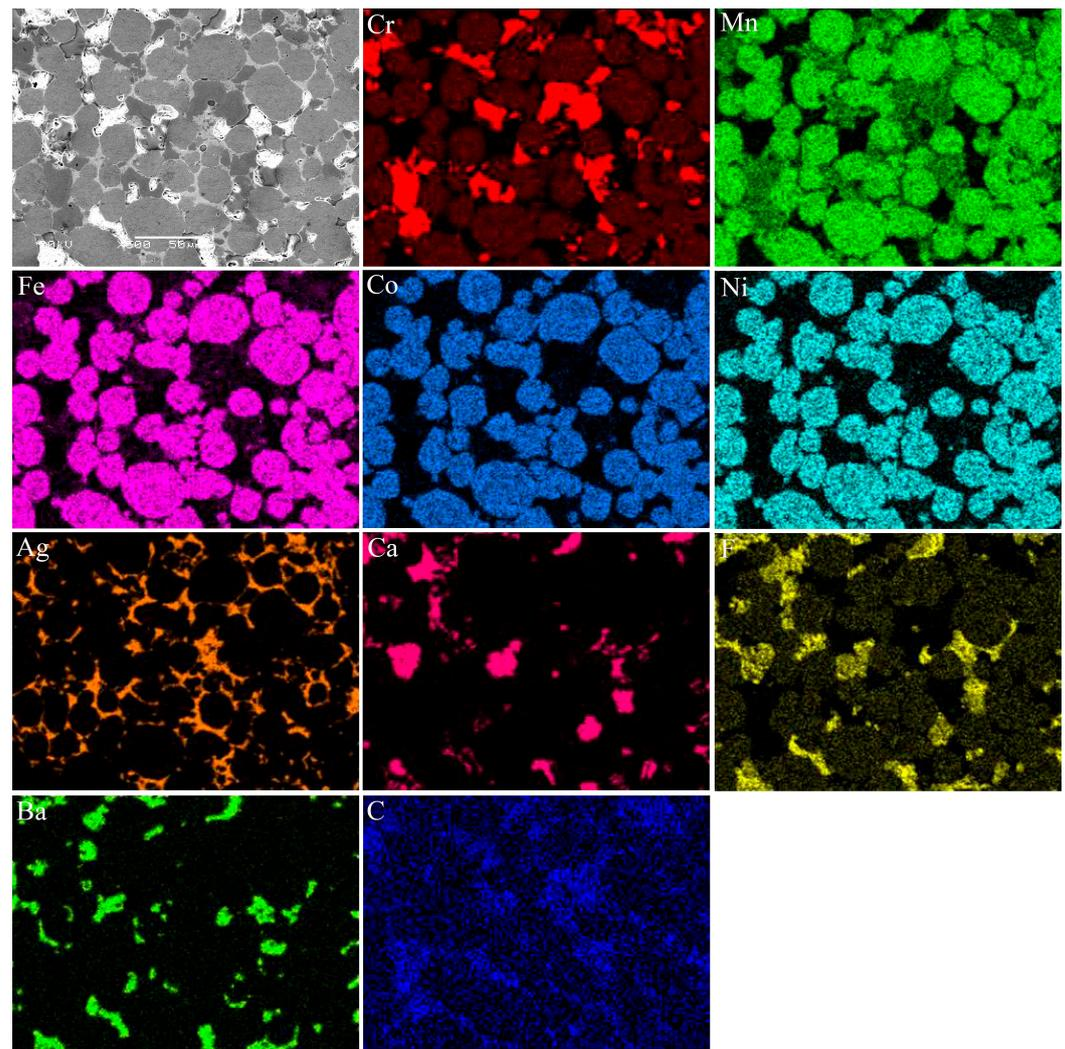
Figure 3. Typical SEM images of the SPSed HEA-15F composites after etching and element distribution.
