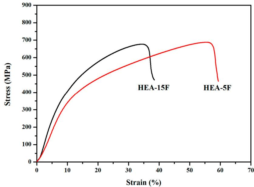
**Figure 4.** The compressive stress–strain curves of the composites at room temperature.
