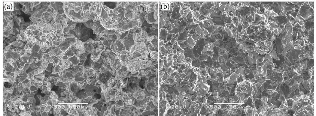
**Figure 5.** SEM images of fracture surfaces of CoCrFeNiMn-Cr<sub>3</sub>C<sub>2</sub>-Ag-CaF<sub>2</sub>/BaF<sub>2</sub> composites: (a) CoCrFeNiMn-Cr<sub>3</sub>C<sub>2</sub>-Ag-5%CaF<sub>2</sub>/BaF<sub>2</sub>, and (b) CoCrFeNiMn-Cr<sub>3</sub>C<sub>2</sub>-Ag-15%CaF<sub>2</sub>/BaF<sub>2</sub>.
