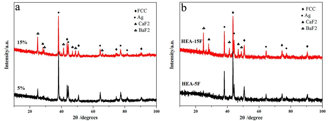
**Figure 1.** The XRD patterns of the mixed raw powders and the SPSed composites: (a) the mixed raw powders and (b) the SPSed composites.
