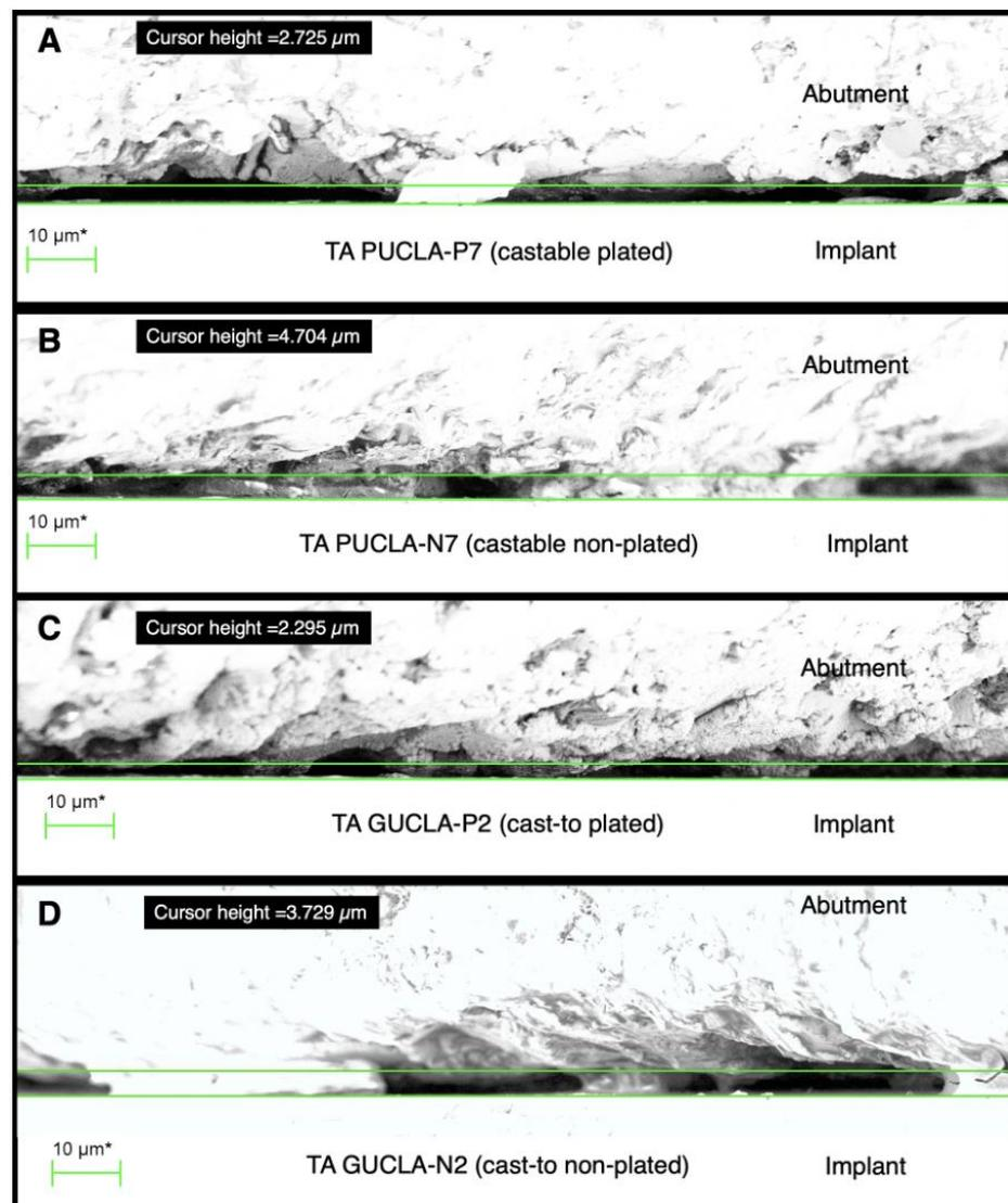
**Figure 6.** Sections of external perimeter micro-gap profiles for examples of the 4 different TA types: (A)—PUCLA-P7, (B)—PUCLA-N7, (C)—GUCLA-P2, (D)—GUCLA-N2. Note the surface asperities, which are in intimate contact with the implant surface. The average “gap” set by the cursor is  $<5 \mu\text{m}$  for the 4 TAs.
