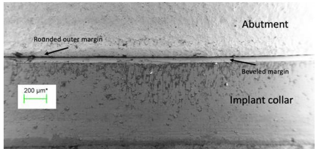
**Figure 4.** The external perimeter of the implant/abutment junction at 100 times magnification, illustrating the beveled margin on the implant and the rounded outer edge of the abutment. The bounded green line in the box is a linear reference of the magnification scale.
