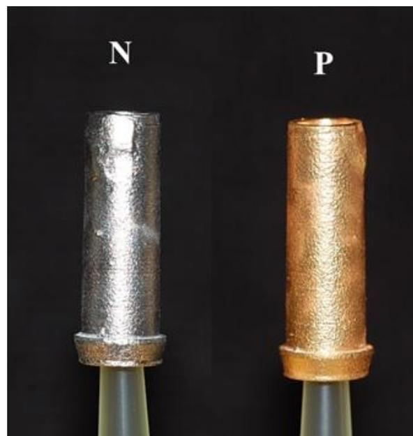
**Figure 1.** Samples of the PUCLA abutments (N = non-plated, P = plated).
