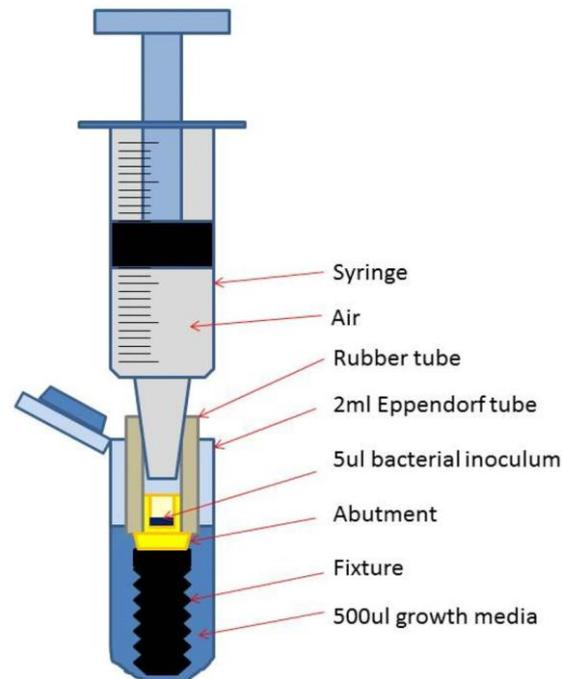
**Figure 2.** Schematic drawing of a test assembly (TA) placed in the Eppendorf tube with added growth medium.
