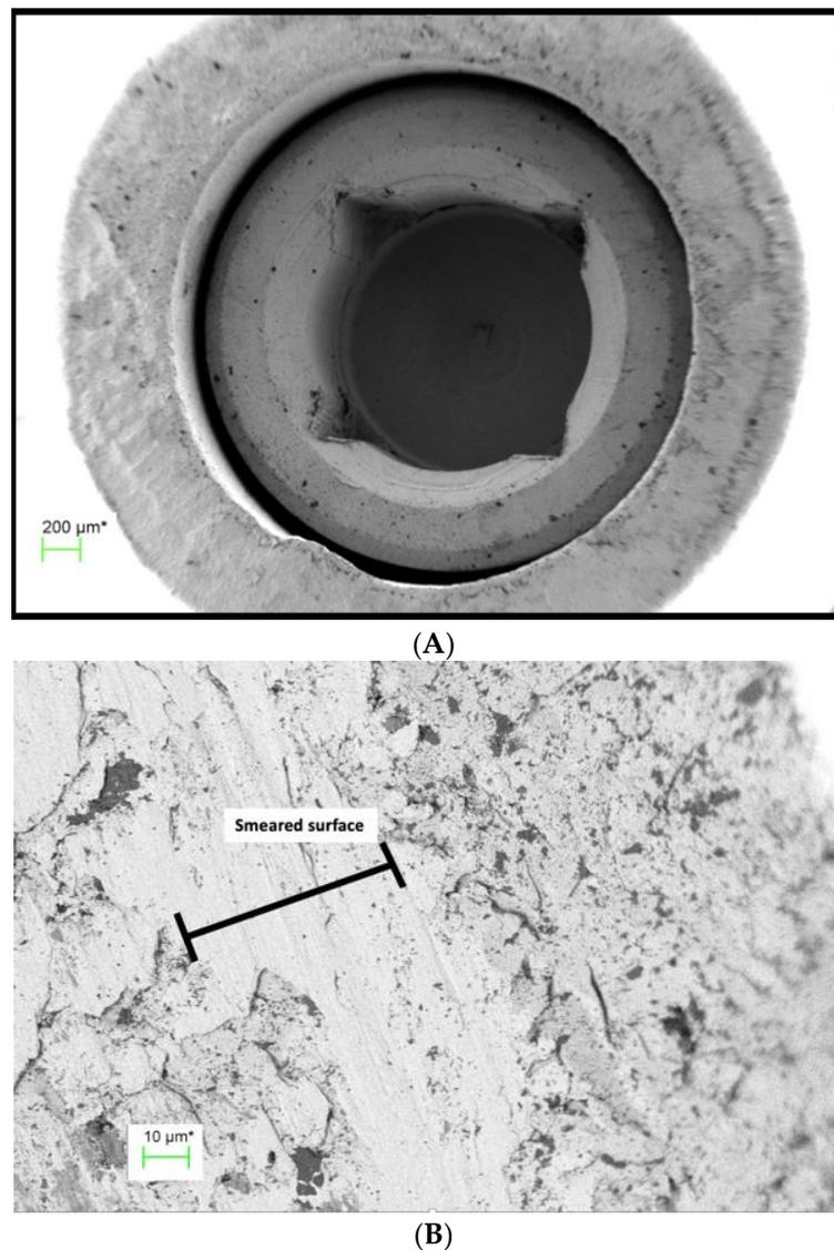
**Figure 9.** (A) Abutment fitting surface of TA PUCLA-N5 at 60× magnification showing a region of smeared surface. (B) Higher magnification of abutment fitting surface of TA PUCLA-N5 at 1580× magnification showing a region of smeared surface.
