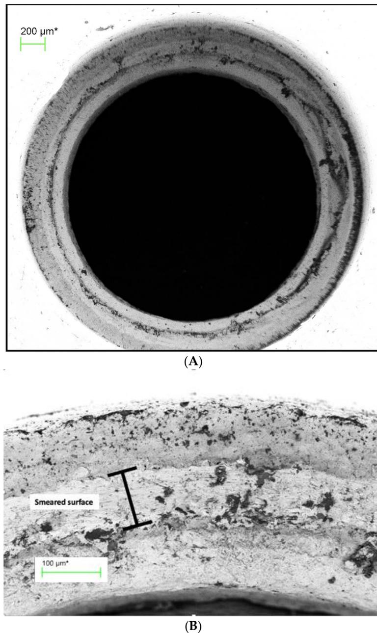
**Figure 7.** (A) Abutment screw seat of TA PUCLA-N5 (70×). (B) Higher magnification (454×) of a section of the screw seat of the abutment of TA PUCLA-N5.
