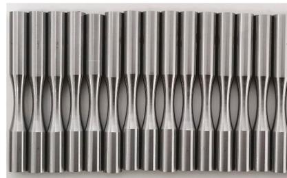
Figure 10. Hourglass-shaped specimen.
