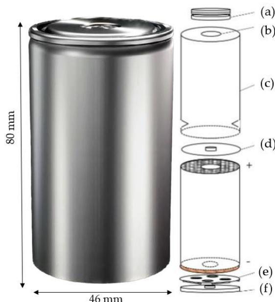
**Figure 20.** Tesla 4680 battery: (a) Pole cylinder, (b) front opening, (c) can, (d) positive collector plate, (e) negative collector plate and (f) cover plate.
