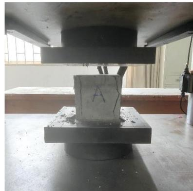
(a) Mechanical properties test of concrete
