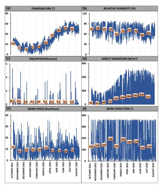
**Figure 2.** Hourly average weather parameters recorded throughout the testing period, including (a) Temperature, (b) Relative Humidity, (c) Precipitation, (d) Direct Radiation, (e) Wind Speed, and (f) Wind Direction. The labels represent monthly average values for each parameter.
