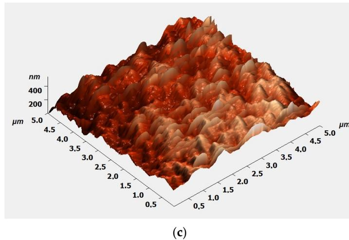
**Figure 4.** 3-D surface models of phosphate coatings: (a) From a modified solution; (b) From a solution with the addition of zinc nitrate; (c) From a solution with the addition of calcium nitrate.
