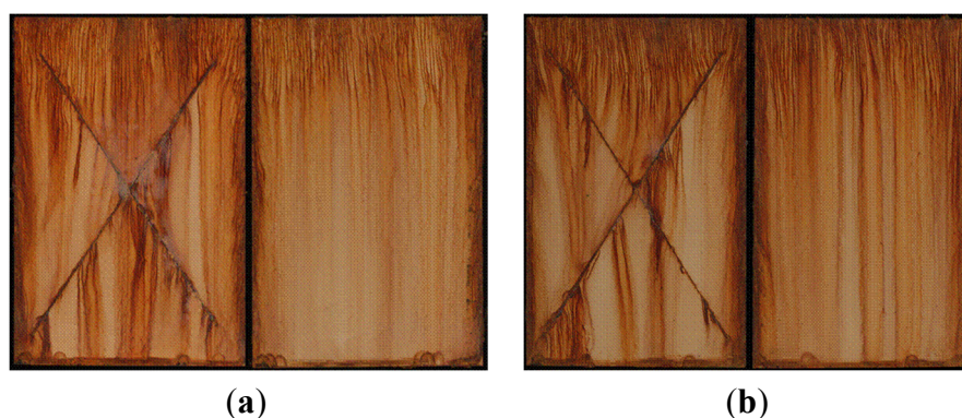
Figure 5. DOD-P-15328D coated on (a) as-received and (b) grit-blasted 4130 steel coupons with MIL-DTL-53022 primer and MIL-DTL-64159 topcoat after 432 h of NSS exposure.
