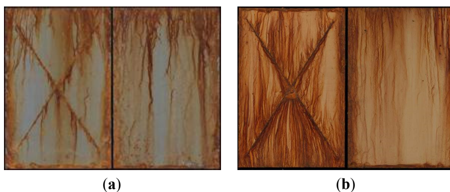
Figure 5. DOD-P-15328D coated on (a) as-received and (b) grit-blasted 4130 steel coupons with MIL-DTL-53022 primer and MIL-DTL-64159 topcoat after 432 h of NSS exposure.
