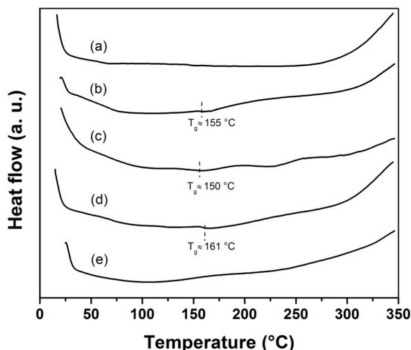
**Figure 6.** DSC thermograms of SR (a), SR-g-(NVCL-co-NVIM) 75% graft (b), poly(NVCL-co-NVIM) (c), SR-g-NVIM 90% graft (d), and SR-g-NVCL 29% graft (e).
