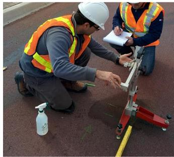
**Figure 3.** Pavement friction assessment by using a British Pendulum tester (BPT).
