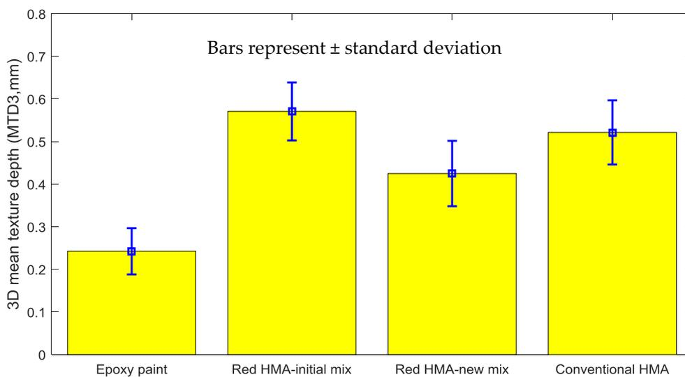
Figure 5. Pavement 3D mean macrotexture depth of tested sections.
