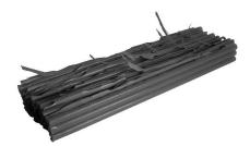
Figure 8. Tubular plastic wood model after a serrated tool was drawn across its surface.
