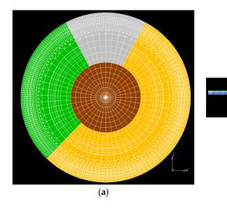
Figure 3. Developed finite element model of the PC wheel: (a) front view and (b) side view.
