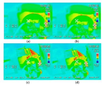
**Figure 8.** Measured temperatures on the substrate: (**a**) front board for second part; (**b**) front board for third part; (**c**) back board for second part; (**d**) back board for third part of generated heat.
