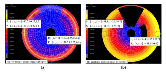
Figure 9. Selected points for extracting thermal results: (a) on phosphor layer and (b) on substrate.
