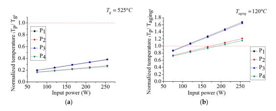
Figure 10. Normalized temperature of wheels for different laser powers: (a) GP wheel and (b) SP wheel.
