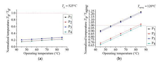
**Figure 13.** Normalized temperature of wheels under different operating temperatures: (**a**) GP wheel and (**b**) SP wheel.
