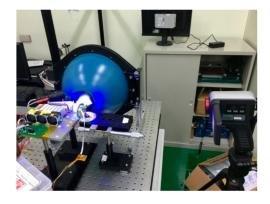
Figure 6. Measurement setup for modified heat coefficient.
