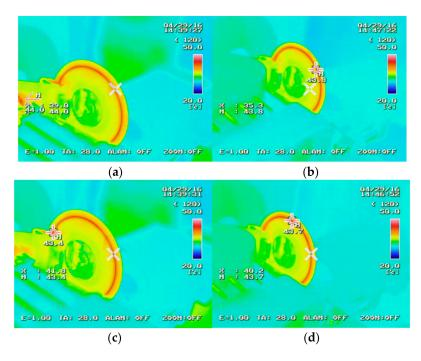
**Figure 7.** Measured temperatures on the phosphor layers: (**a**) front board for first part; (**b**) front board for third part; (**c**) back board for first part; and (**d**) back board for third part of generated heat.
