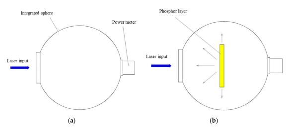
**Figure 5.** Measurement setup for heat absorption coefficient of phosphor: measurement of (**a**) optical laser power and (**b**) converted laser power.
