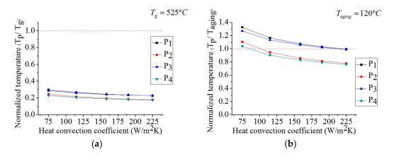
**Figure 14.** Normalized temperature of wheels with different heat convection coefficients: (**a**) GP wheel and (**b**) SP wheel.
