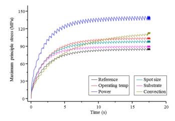
Figure 17. The flow of maximum principle stress at point P<sub>2</sub>.
