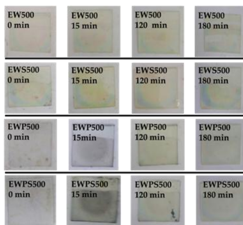
Figure 2. Changes of the appearance of the EW500, EWS500, EWP500, and EWPS500 films (annealed at 500 °C) as the annealing time increased. The color changed from transparent to grey and finally turned transparent again only in the samples EWP and EWPS (PEO-doped), which indicated the carbonization of PEO at high temperature.
