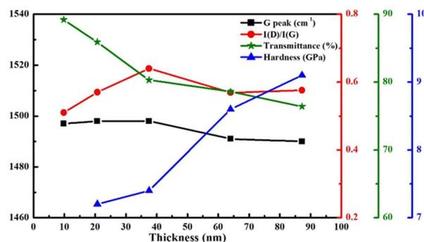
**Figure 8.** The analysis of DLC properties and transmittance in the different thickness of SiO<sub>x</sub>:DLC films. (RF bias = 400 V, DC power = 50 W, CH<sub>4</sub> = 12.5 sccm, HMDSO = 0.9 sccm).
