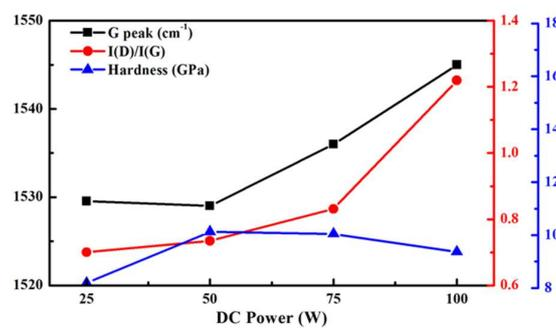
**Figure 3.** The analysis of DLC properties in the DC power range of 25–100 W with RF bias of 400 V. (CH<sub>4</sub> = 15 sccm, Thickness = 150 ± 10 nm).
