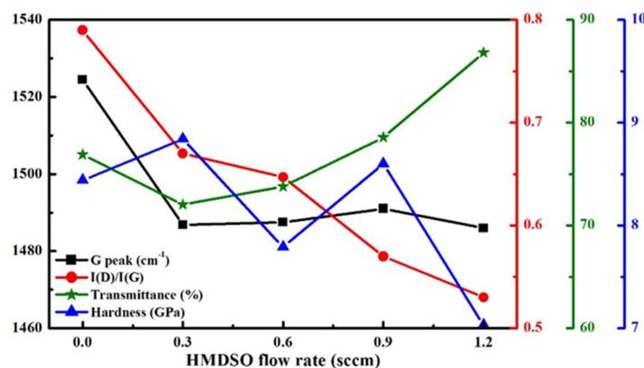
**Figure 6.** The analysis of DLC properties and transmittance at the different HMDSO flow rates. (RF bias = 400 V, DC power = 50 W, CH<sub>4</sub> = 12.5 sccm, thickness = 65 ± 5 nm).
