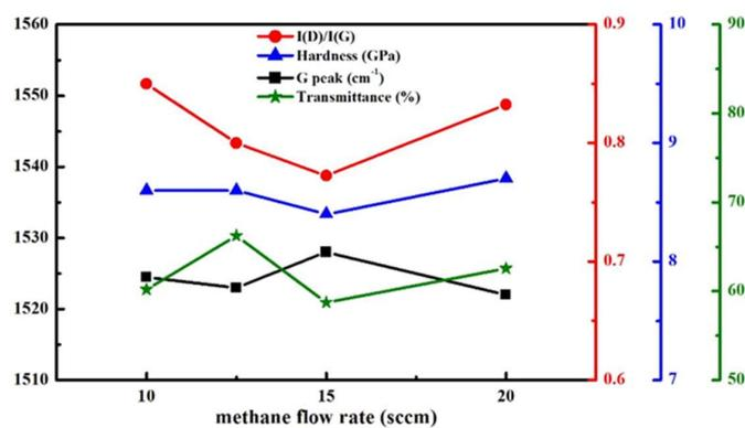
**Figure 4.** The analysis of DLC properties and transmittance at the different CH<sub>4</sub> flow rates with RF bias of 400 V and DC power of 50 W. (thickness = 135 ± 10 nm).
