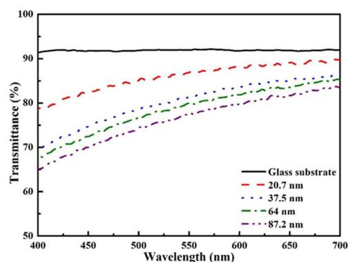
**Figure 9.** The transmittance spectra of SiO<sub>x</sub>:DLC films with different thickness. (RF bias = 400 V, DC power = 50 W, CH<sub>4</sub> = 12.5 sccm, HMDSO = 0.9 sccm).
