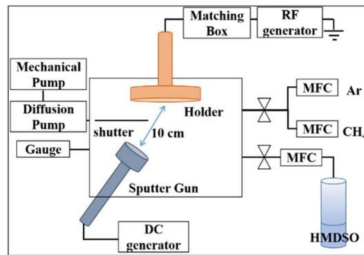
**Figure 1.** Schematic diagram of the apparatus used for deposition of SiO<sub>x</sub>: diamond-like carbon (DLC) films. Radio frequency (RF), hexamethyldisiloxane (HMDSO), mass flow controller (MFC).
