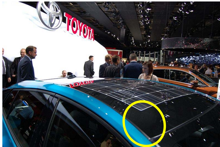
Figure 1. Picture of the car-roof of Solar-Prius, a PHV product of Toyota Motor mounting 180 W of high-efficiency crystalline Si cells. Note that the area with significant curvature is not covered by the solar cells (like inside the yellow circle) [47].
