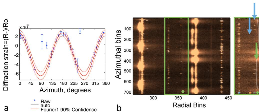
**Figure A2.** Strain analysis and fitting challenges for transformed Debye rings: (a) fitting challenges for strain response with bond coat overlap over alumina peak, with representations of in plane (e22) and out of plane (e11) strain data; and (b) examination of transformed Debye rings with precipitates obscuring oxide layer ring. Secondary peaks marked in blue interfere with faint TGO peak marked in green.
