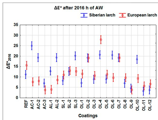
**Figure 5.** Total colour difference of coating systems applied to European and Siberian larch after 2016 h of artificial weathering evaluated as 95% two-side confidence intervals. The Tukey HSD test shows that the differences in the analysed values were statistically significant ( $p$ -value < 0.05) for coating systems AC-1, AC-2, AL-1, AL-2, SL-3, OL-4, OL-6 and OL-10.
