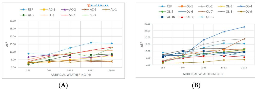
**Figure 3.** The total colour difference of acrylate, alkyd, synthetic (A) and oil-based (B) coating systems applied to European larch during artificial weathering lasting 168 h, 504 h, 1512 h and 2016 h.
