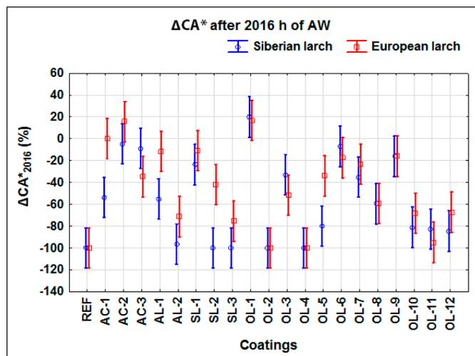
**Figure 8.** Changes in the water contact angle on the tested coatings in percentages after 2016 h of artificial weathering evaluated as 95% two-side confidence intervals. The Tukey HSD test shows that the differences in the analysed values were statistically significant ( $p$ -value < 0.05) for coating systems AC-1 and SL-2.
