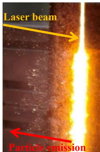
**Figure 4.** Emission of particles from the irradiated surface produced by thermal stresses induced in the black granite.
