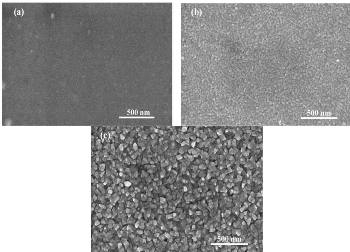
**Figure 3.** SEM images of AlSb:Zn thin films deposited at different substrate temperatures: (a) 300 °C; (b) 350 °C; (c) 400 °C.
