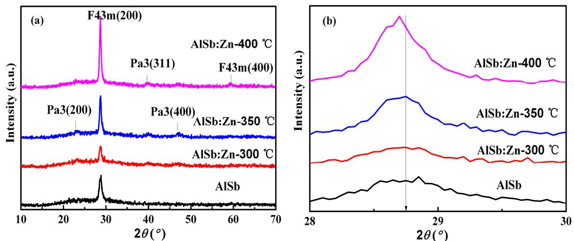
**Figure 2.** (a) Full scale and (b) enlarged scale XRD patterns of AlSb:Zn thin films deposited at different substrate temperatures.
