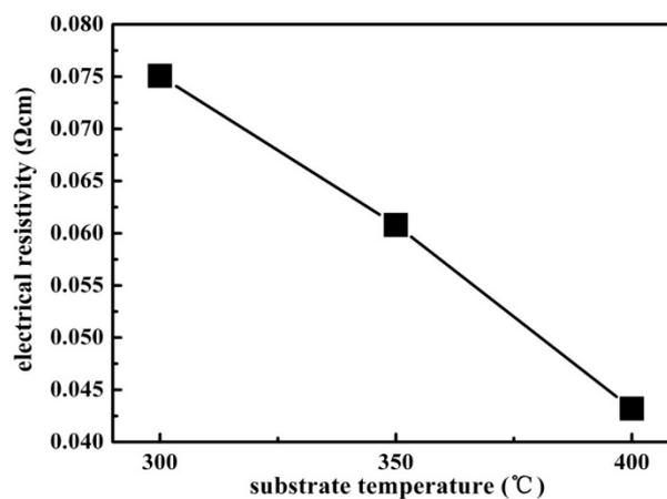
Figure 5. The electrical resistivity of AlSb:Zn thin films deposited at different substrate temperature.
