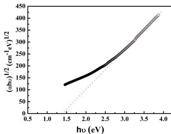
Figure 6. Plot of  $(\alpha h\nu)^{1/2}$  versus  $h\nu$  profile of a representative AlSb:Zn film deposited at 400 °C.
