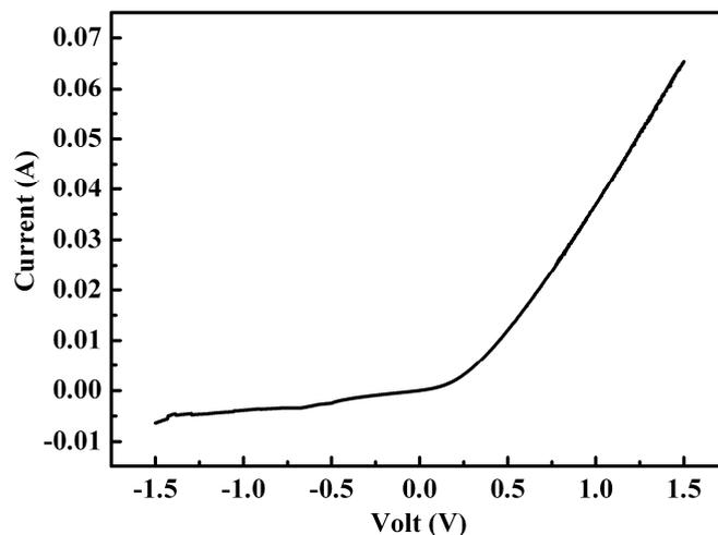
Figure 10. Dark  $I$ - $V$  curve of a ZnS/AlSb:Zn thin film solar cell.
