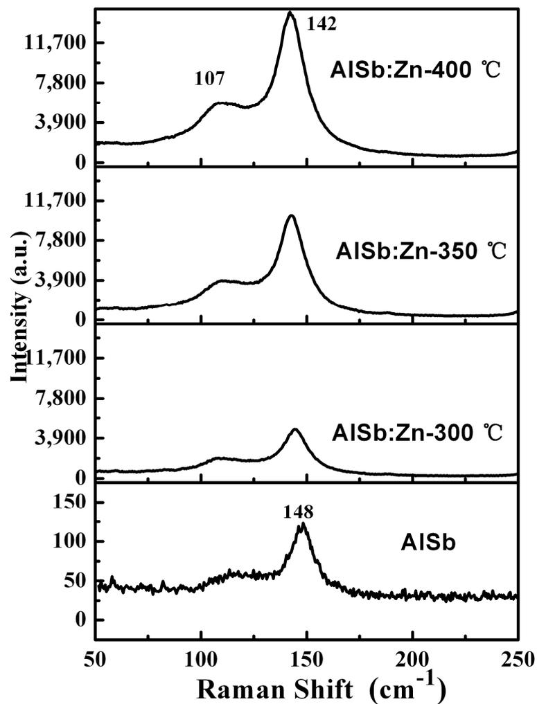
Figure 4. Raman spectra of AlSb:Zn thin films deposited at different substrate temperatures.
