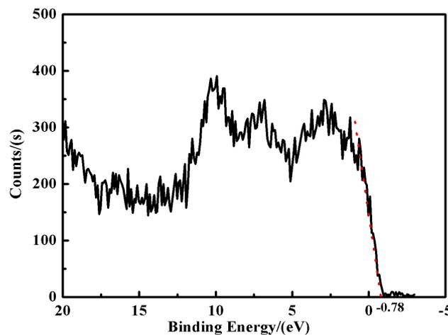
Figure 7. The valence band spectrum of a representative AlSb:Zn film deposited at 400 °C.
