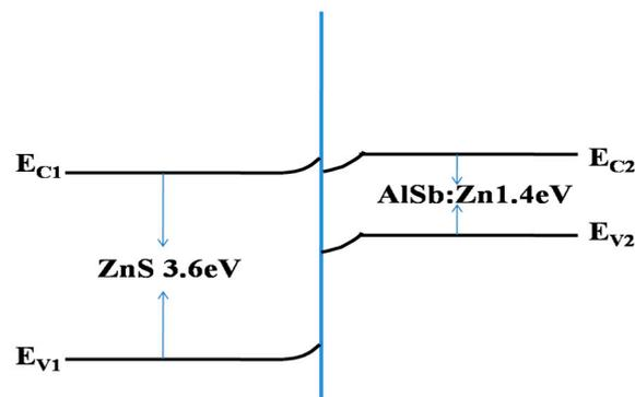
**Figure 9.** The energy band of the ZnS/AlSb:Zn heterojunction.
