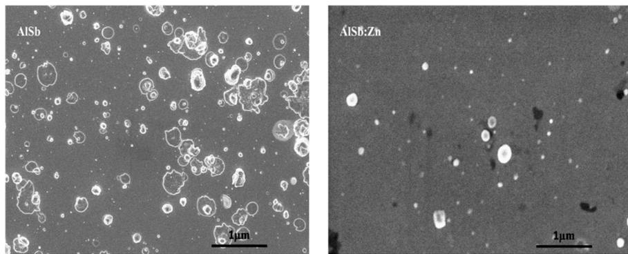
**Figure 8.** SEM images of AlSb and AlSb:Zn thin films stored in a vacuum chamber for 48 h.
