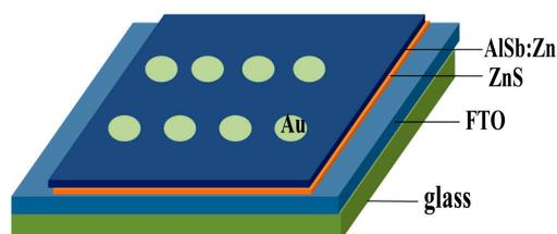
Figure 1. Structure of AlSb-based solar cells.
