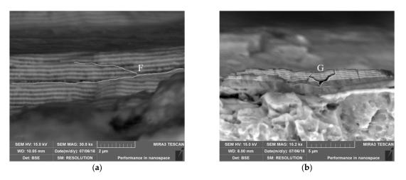
Figure 7. (a) Crack deflection and (b) crack branching of the TiN/ZrN multilayer coating.
