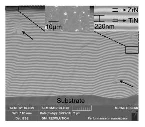
Figure 3. Sectional morphologies of the TiN/ZrN multilayer coatings.
