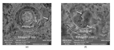
**Figure 6.** SEM micrographs of uncoated and coated samples after 60 g erosion testing: (**a**,**b**) are the uncoated sample, (**c**) is the erosion area, (**d**) is an enlargement of the white frame in (**c**), and (**e**,**f**) are an enlargement of the failed area with droplets defects (D) and stress concentration defects (E) during the coating process.
