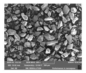
Figure 1. SEM micrographs of the erosion sand.
