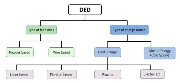
Figure 1. Classification of Directed Energy Deposition (DED) systems.
