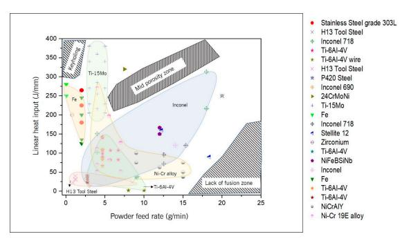
**Figure 7.** Optimal processing regions for Ti-6Al-4V, Inconel 690-718, Ni-Cr based alloys, Fe, H13 tool steel, and Ti-15Mo alloy, along with the unsuitable processing zones, as compiled in Table 5.
