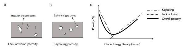
**Figure 6.** Schematic of: (a) Lack of fusion porosity (interlayer porosity), (b) keyholing porosity (intralayer porosity), and (c) the intersection of interlayer and intralayer porosity with respect to global energy density (GED).
