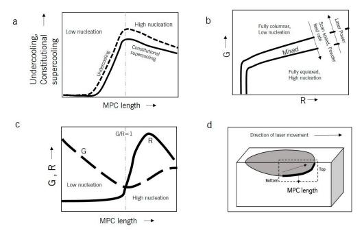
**Figure 4.** The relationships explaining the process maps for G vs. R, derived from [80]; (a) graph of undercooling/constitutional supercooling versus melt pool circumference (MPC) length showing the transition from low nucleation to high nucleation (columnar to equiaxed transition), (b) trend of the columnar to equiaxed transition from the graph of G versus R, (c) variation of the G/R ratio with respect to the MPC length, and (d) the MPC length as defined from the bottom to the top.
