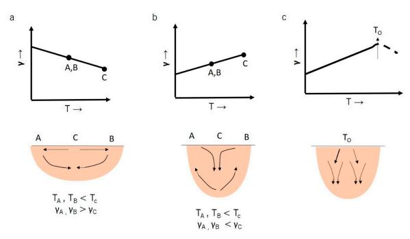
**Figure 3.** Schematic of Marangoni effect using the Heiple–Roper theory of weld pool geometry, depending on the surface tension and temperature of the melt pool, as applicable for DED systems. (a) Melt pool geometry when the surface tension gradient is negative, (b) melt pool geometry when the surface tension gradient is positive, and (c) melt pool geometry when the surface tension gradient shifts from positive to negative.
