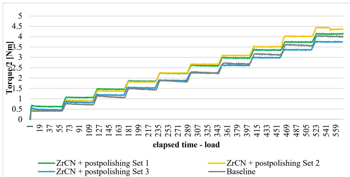
Figure 16. 594A/592A ZrCN + polish post-processing TTR friction test 0–15 kN, 30 rpm.
