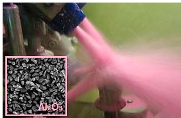
**Figure 1.** Abrasive jet machining process.
